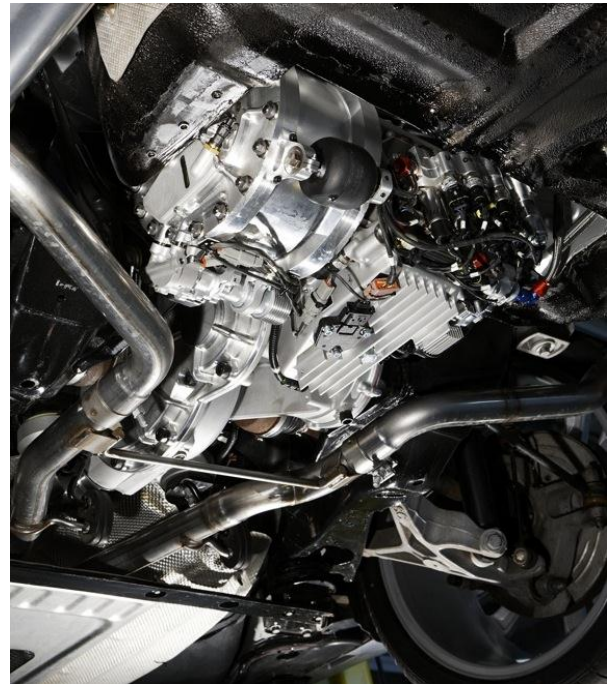
Flybrid flywheel system fitted to Jaguar test car in Flywheel Hybrid System for Premium Vehicles Project
