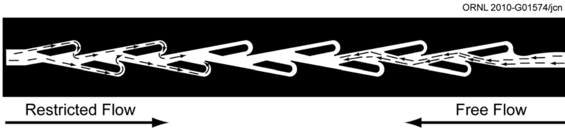
Fig. 1. Tesla flow diode patented in 1920. (US Patent 1,329,559)
