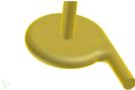
Fig. 10. Typical vortex diode configuration meshed with GAMBIT.
