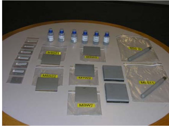
Figure 4 – Samples of amorphous-metal HVOF coatings used for long-term corrosion testing.
