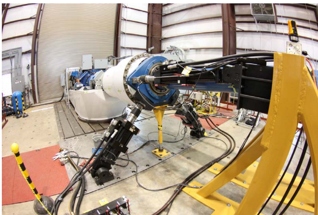
Figure 4. NREL/PIX18952: Non-torque load mechanism in NREL dynamometer.
