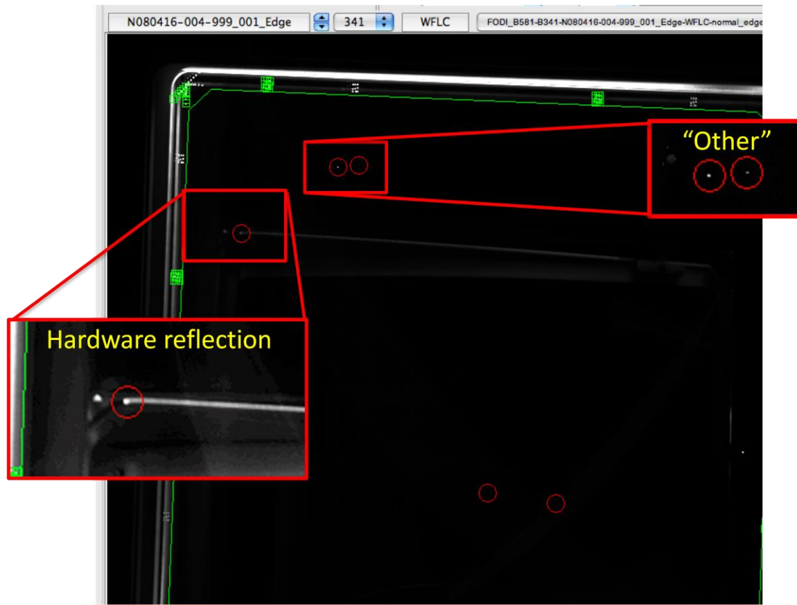
Figure 1: shows an example of a FODI image. Possible damage sites are the small dots identified by a red circle around them. The bright dot at the end of a thin line is a reflection from nearby hardware that was falsely identified by the image analysis software as a possible damage site. The purpose of this study is to automatically distinguish the two by applying machine learning algorithms.
