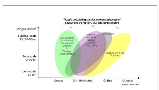
Figure III.1: Time and length scale variation and overlap that is found in building systems. The range of scales that must be captured in simulation and dynamic analysis must drive the creation of new algorithms and mathematical analyses tailored to building systems that capture the thermal and transport phenomena, the controlled dynamics and the uncertainty analysis.
