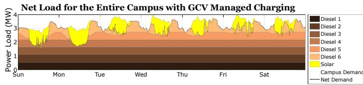
By managing the charge rate relative to change in demand, the load becomes slightly flatter. Minor ripples can be smoothed and sharp drops in demand (or sharp rises in intermittent renewables) can be delayed to mitigate generator ramp times.
