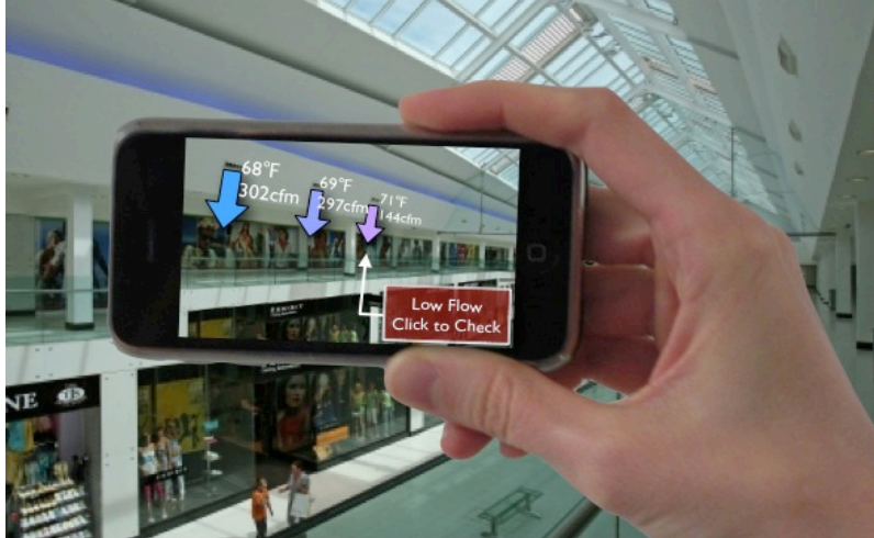
Figure 66. Mockup of augmented reality use case for variable-air volume box diagnostic (Source: NREL)
