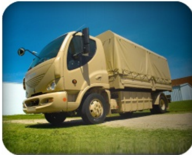
Figure 39. The Smith Electric Newton All-Electric Truck, upfitted into one of many different configurable options (Courtesy of Smith Electric Vehicles, reprinted with permission)
