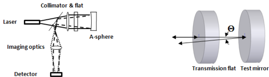
Figure 11. Configuration for measuring focus mirrors with minimum interference cavity path length and calibrated optics.
