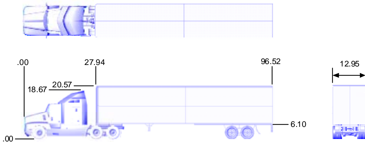
Figure 2: Three-view drawing of baseline tractor-trailer configuration (measurements in cm). Note height mismatch between tractor and trailer due to inaccuracies in the publicly available CAD geometry.
