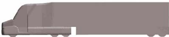
Figure 5. "GTS" Configuration of the GCM, with Full Gap Fairing and Trailer Belly Box.
