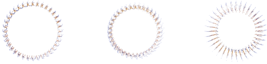
Figure 7.2: Ray-plane intersections for the Dinosaur dataset, at planes Z = -1 (left), Z = 0 (middle) and Z = 5 (right).
