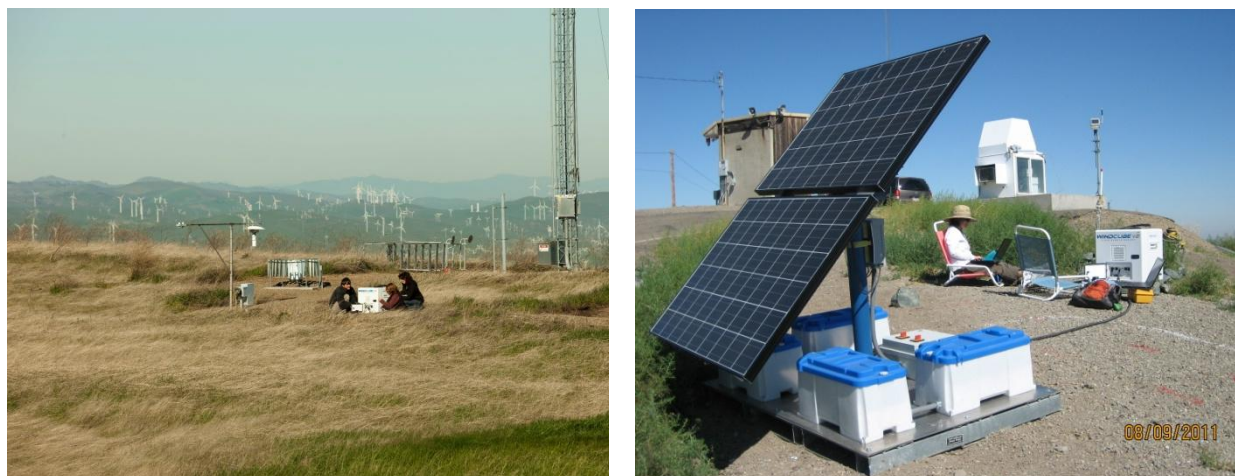
Figure A2: The project team downloading data from (left) the LIDAR co-located with the tall meteorological tower at the East Observational Point (EOP) and (right) the LIDAR near the lightning detector upwind of the flux tower. Both systems are fully equipped to run off of solar power. Elevations are 387 m, 387 m, and 398 m, respectively, for the tall meteorological tower, co-located LIDAR at the EOP, and the LIDAR near the lightning detector.
