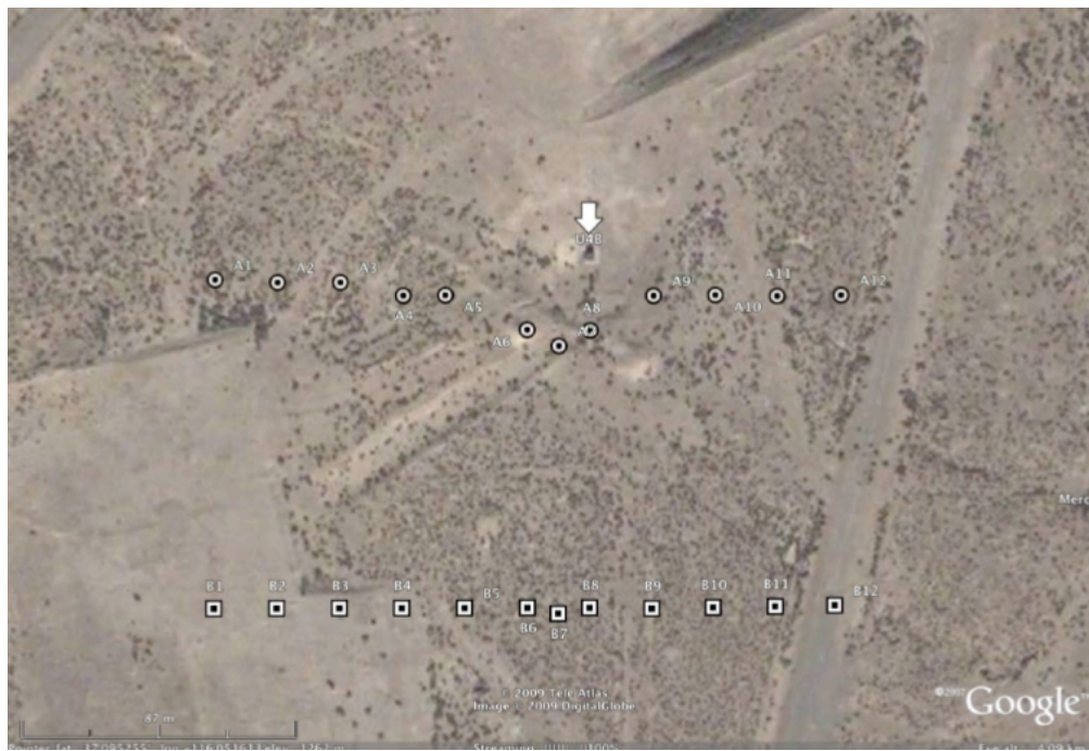
Map showing locations of vertical seismometers (squares) emplaced for the passive seismic experiment. Spacing is about 50 meters. The southern control line (line B) is located 150 m south of line A. The white arrow marks ground zero of event U4a.
