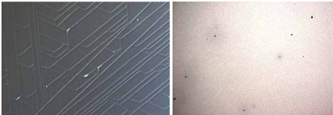
Figure 22. Surface morphology of CdZnTe after In diffusion: (left) cracks on sample D10056; (right) no cracks on sample D10062.
