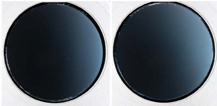
Figure 20 p-CdZnTe sample D10071 (left) and n-CdZnTe/p-CdZnTe sample D10088 (right) grown on Si(211).
