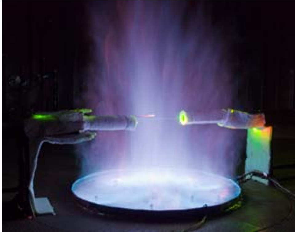
Figure 9. Photograph of a 2-m diameter methanol fueled pool fire.
