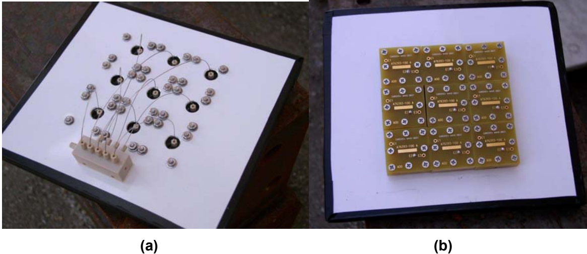
Figure 4. a) Backside photo of 9-plex FR4 array showing gas fill capillaries and Manifold, b) Front side photo of same FR4 array. No electronic connections are shown since tests were done without devices energized.
