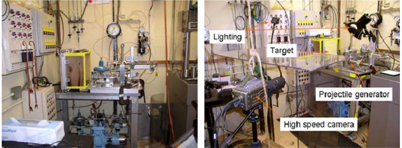
Figure 10. a)High pressure test lab, SNL Livermore, b)Overview of projectile impact test set-up.
