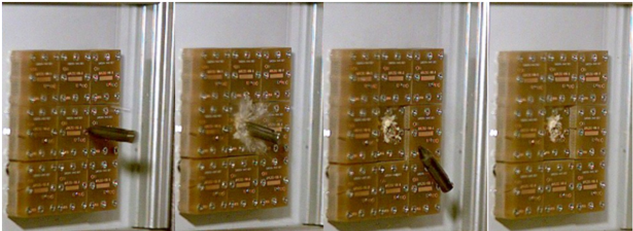
Figure 15. Successive images of projectile impacting array of nine FR4 pressurized devices. Devices were bolted to the support plate.
