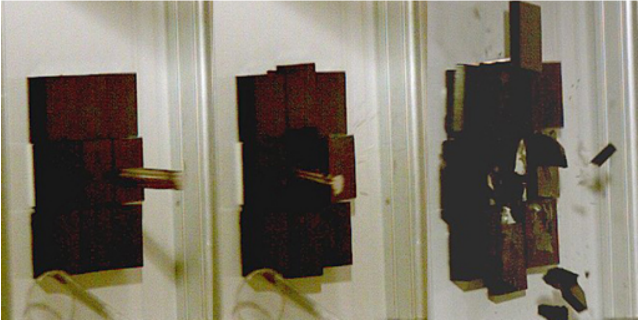
Figure 19. Successive images of projectile impacting array of nine pressurized Parmax devices.
