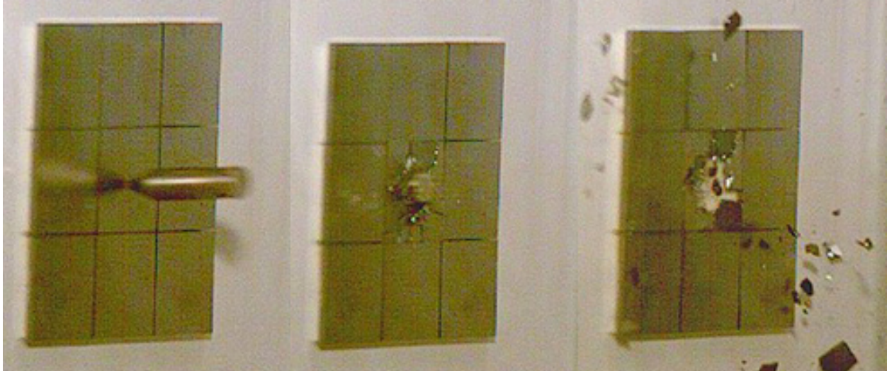
Figure 17. Successive images of projectile impacting array of 9 2x2 silicon devices.
