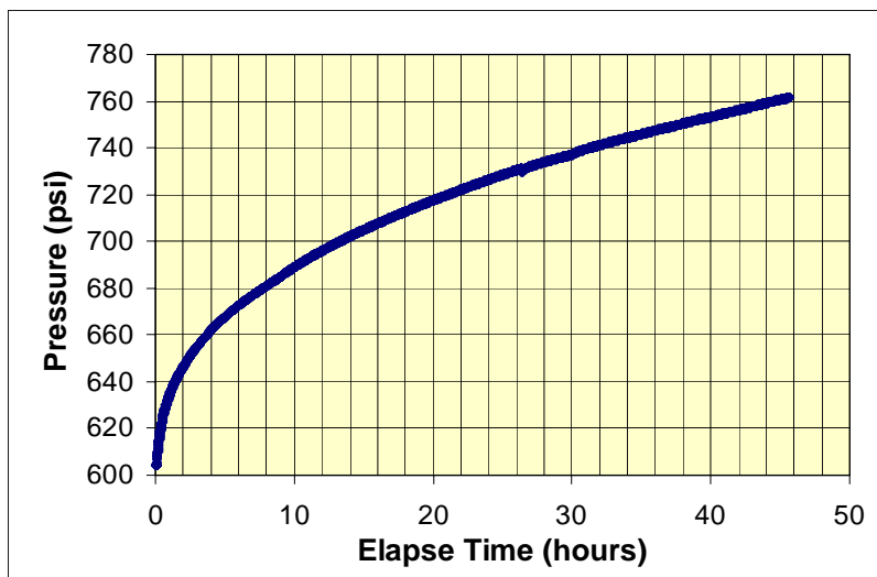
Figure 5.1.4: Bottom hole pressure build-up during water injection into Colliver #7 at a rate of 450 bbl/D(71.5 m 3 /d).
