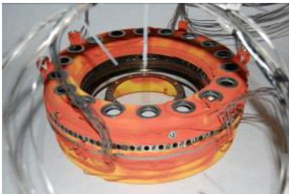
Figure 2.5.3 Advanced CMC combustor after rig test.
