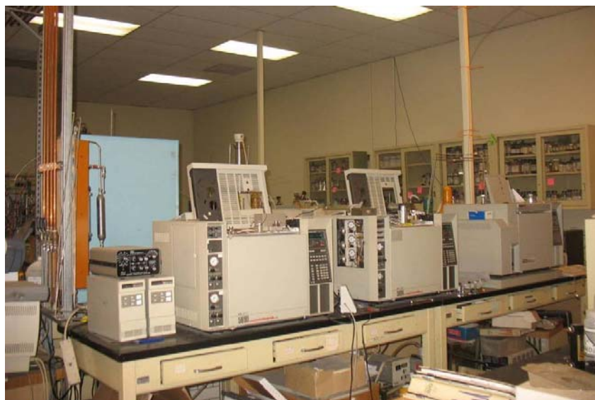
Figure 1 Series of GC/LC equipped with FID, TCD, and ECE detectors to analyze the full-spectrum of the gas products
