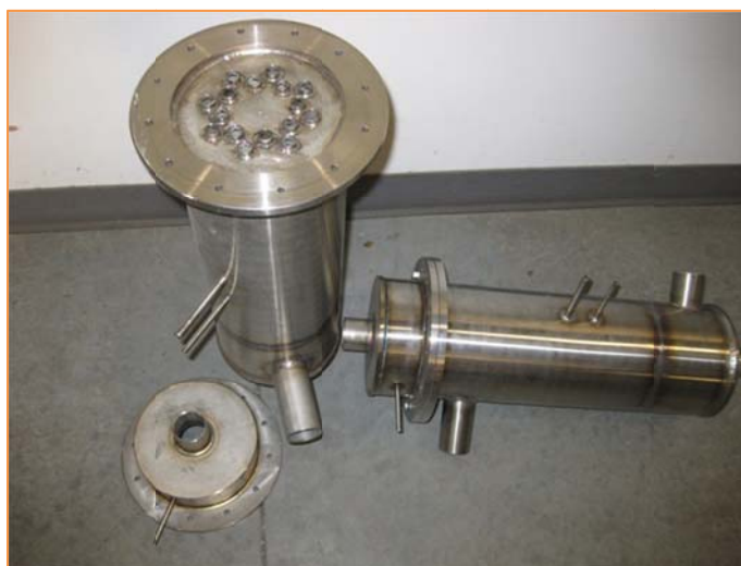
Figure 158. Two tailgas-fired process heaters packed with catalysts
