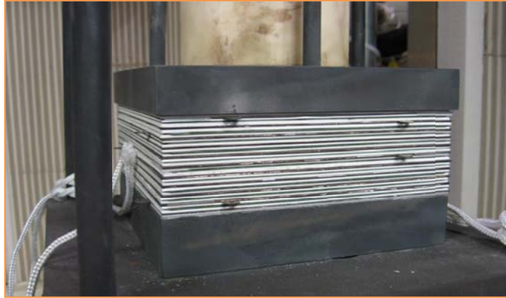
Figure 125. A photograph of a 10-cell stack assembly ready for testing. Each cell had 100 cm 2 active area and attached with a voltage lead,
