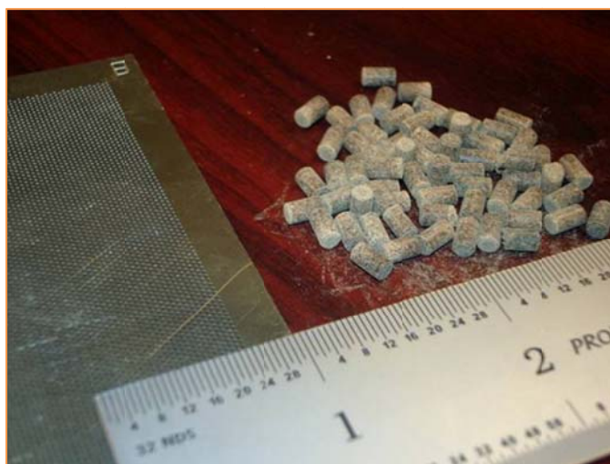
Figure 159. Photograph of the catalyst material used in the tailgas-fired process heaters, along with the micro-perforated SS foil used as the air diffuser
