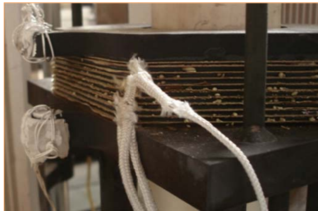
Figure 137. Photograph of the 10-cell hybrid stack (7-SOFEC & 3-SOFC) after testing
