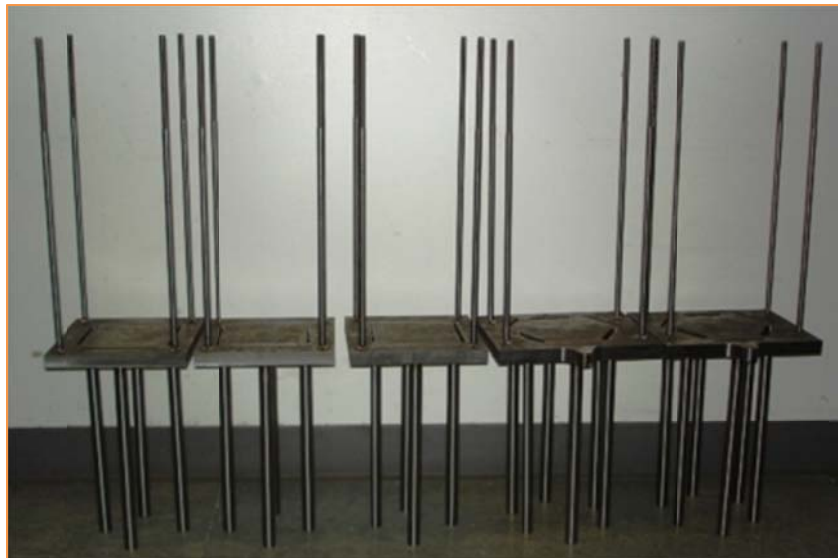
Figure 151. Photograph of five sets of compression hardware machined for modular stacks (the missing one was installed in test station already)
