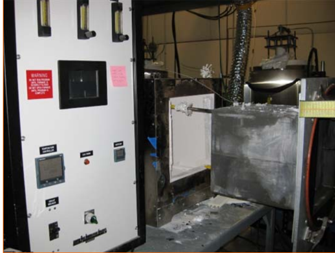
Figure 150. Photograph of the retort furnace used for fabricating interconnects
