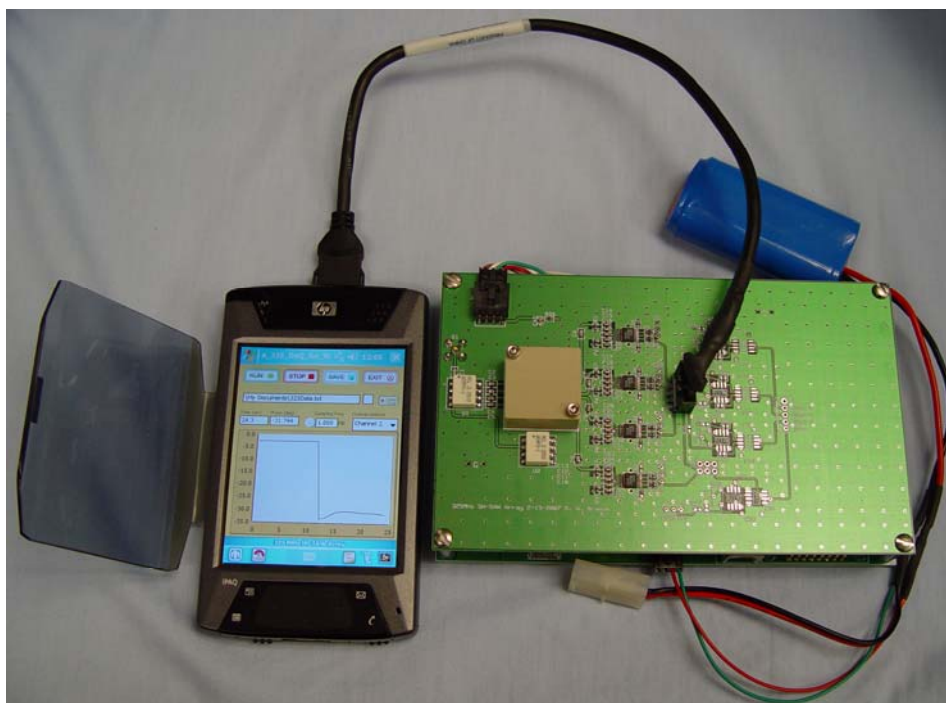
Fig. 10 SH-SAW Four channel phase detection system connected to a PDA NI CF6004 DAQ card. The sample rate was 1k with a phase resolution of 0.01^\circ
