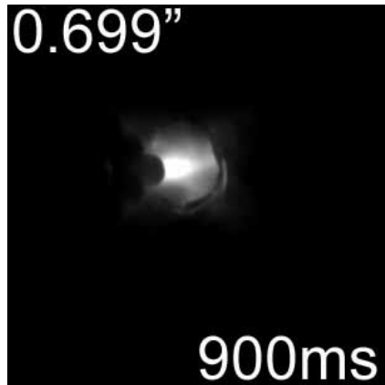
Figure 58. Larger hole associated with severe charge transfer level.
