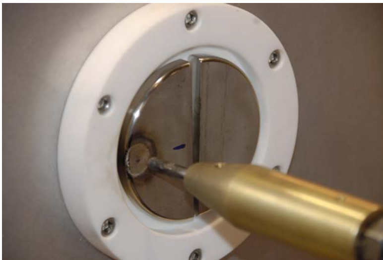
Figure 178. The electrode of the SLS and damage caused to the electrodes by the continuing current.
