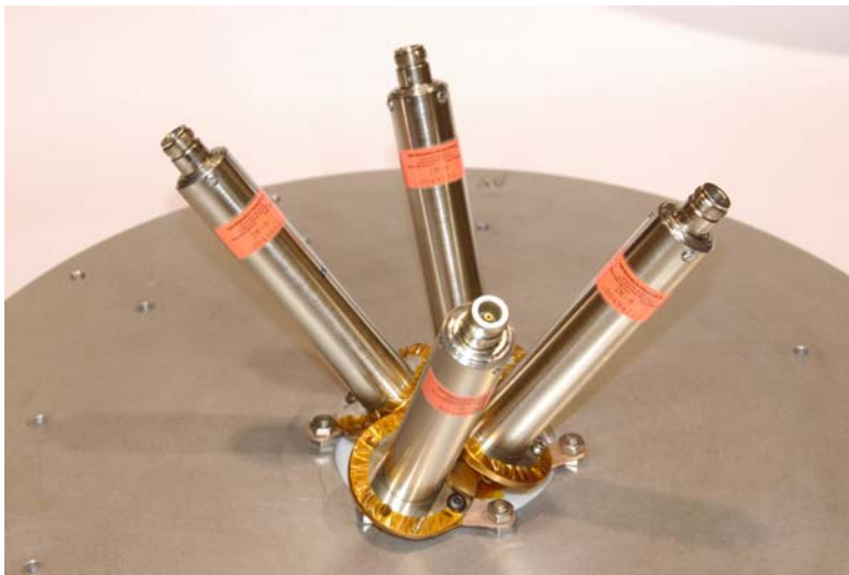
Figure 187. CVRs connected to each of the rings of the probe.
