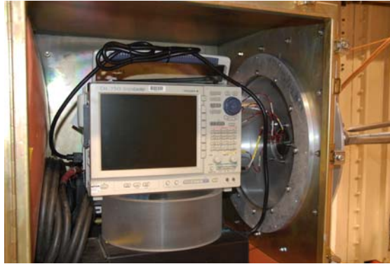
Figure 46. Screen box for housing scope to record multichannel responses of the groove probe.
