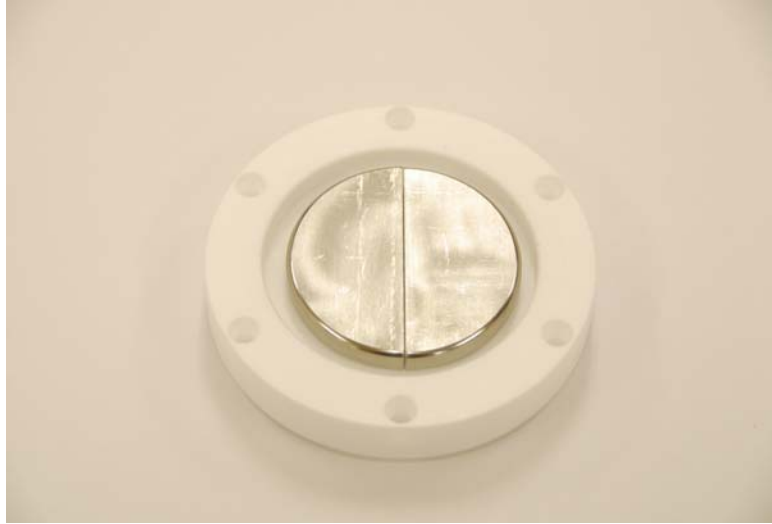
Figure 175. Front of two “D” electrodes for measuring plasma radius.
