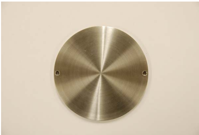
Figure 201. Front side of groove probe.
