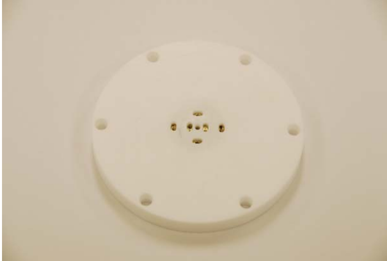
Figure 186. Back view of the ring electrodes of the probe.
