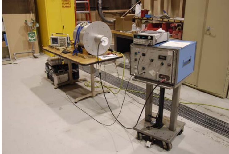
Figure 140. Velonex pulser in foreground with trigger unit on top. Measurement section in background.
