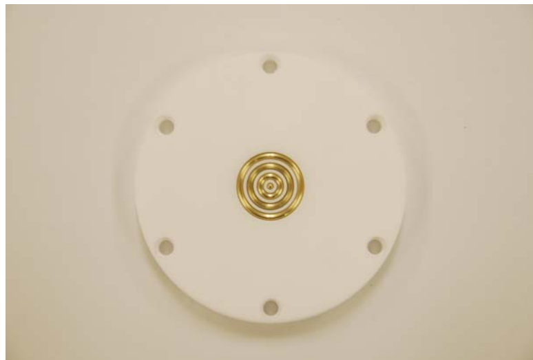
Figure 185. Front view of the ring electrodes. The radii of the ring centers are 1: 0 mm, 2: 4.75 mm, 3: 9.5 mm, 4: 14.3 mm.
