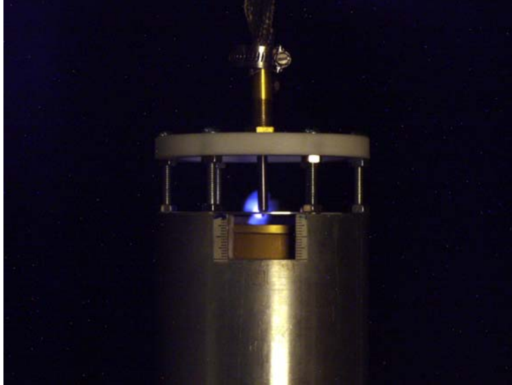
Figure 160. Picture of the case where the electrode is interior to the barrier.
