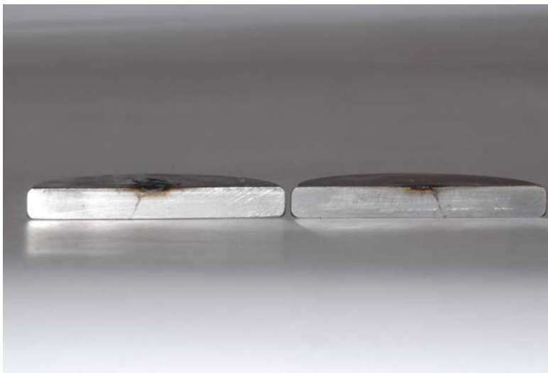
Figure 180. Side view of electrode damage.
