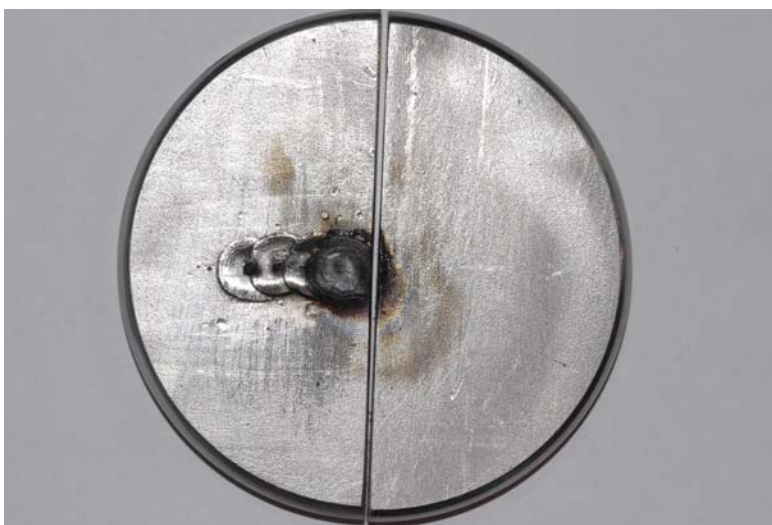
Figure 179. Damage to electrodes from continuing current.
