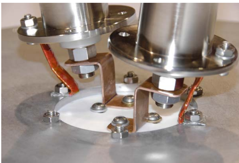
Figure 177. CVR's attached to back of “D” electrodes.
