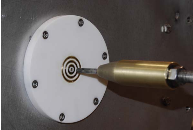
Figure 190. SLS electrode and the ring electrodes of the probe.
