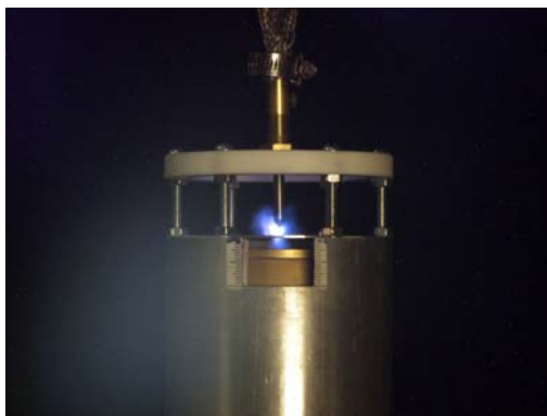
Figure 49. The cathode was positioned exterior to the predrilled barrier hole.
