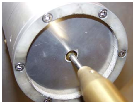
Figure 47. Predrilled hole used for Sandia Lightning Simulator discharge to collector experiment.
