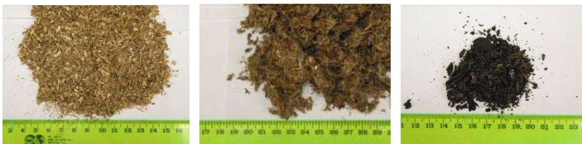
Figure 7. Photographs of dried, chopped corn stover (left), dried solids remaining after SAA treatment of the corn stover (middle), and lignin residue collected by drying the ammonia effluent (right).
