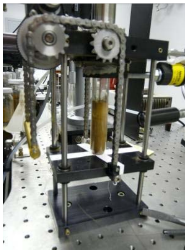
Figure 10. Photograph of custom -designed fine particle feeder for dry coal and biomass samples. For feeding of particularly sticky biomass samples, steel shot can be added to the test tube to help break-up particle aggregates.
