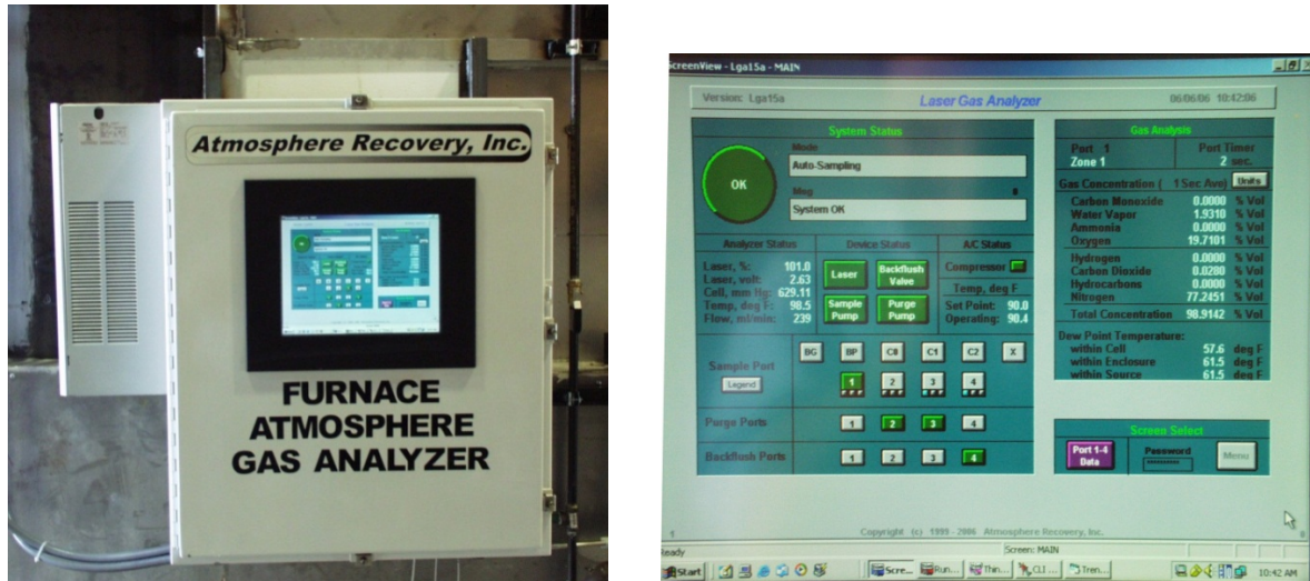
Figure 4-7. Laser Gas Analyzer
