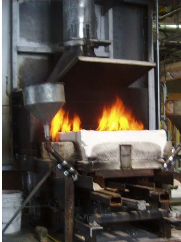
Figure 2-7-6(a). Flame shooting out from the entrance end of LHF when a sample tray was in Zone 1.
