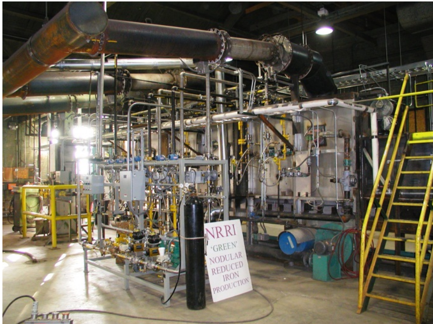
Figure 4-1. Pilot-Scale Linear Hearth Furnace Simulator
