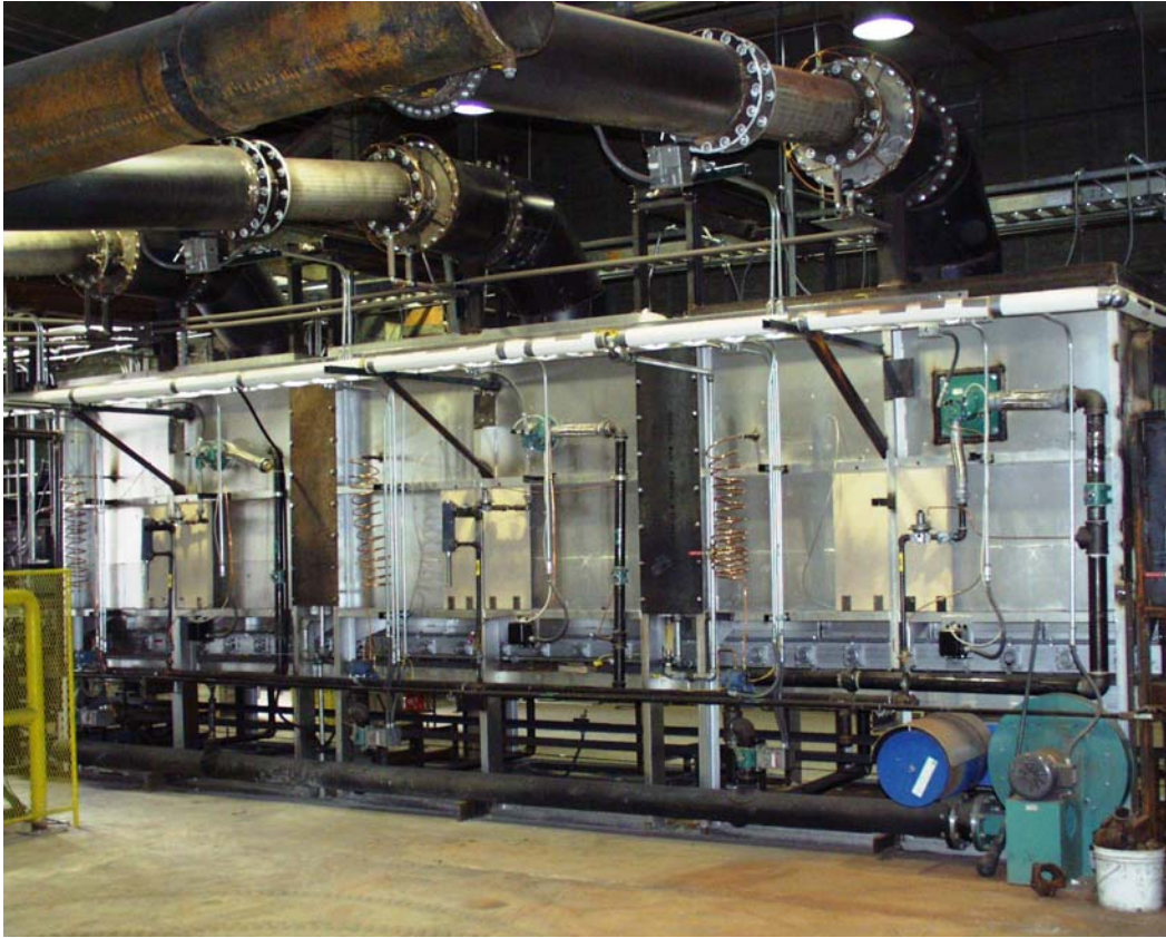
Figure 4-2. Linear Hearth Furnace 3-Zone Configuration
