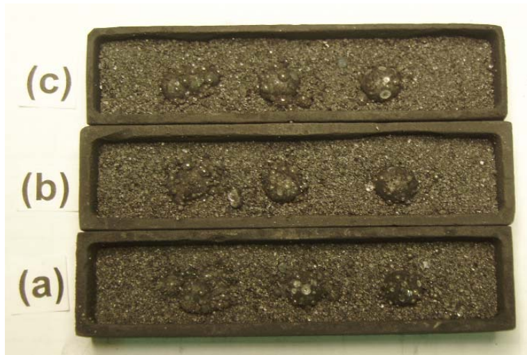
Figure 2-4-11. 2.5g piles of mixtures of 14/20 mesh micro NRI and crushed NRI in the ratios of (75:25) on the left, (50:50) in the middle and (25:75) on the right, placed over 20/100 mesh coke hearth layer, and heated at 1350°C (2462°F) for different periods of time in a N 2 -CO atmosphere.
