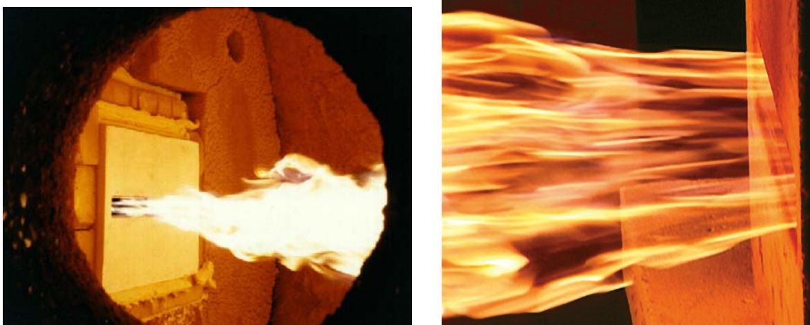
Figure 4-11. Flat flame burner design
