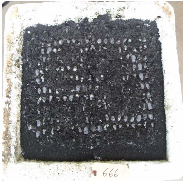
(a) PRB cover layer of 6.8 kg/m 2 (1.4 lb/ft 2 ) (>50% of briquettes exposed to furnace atmosphere)
