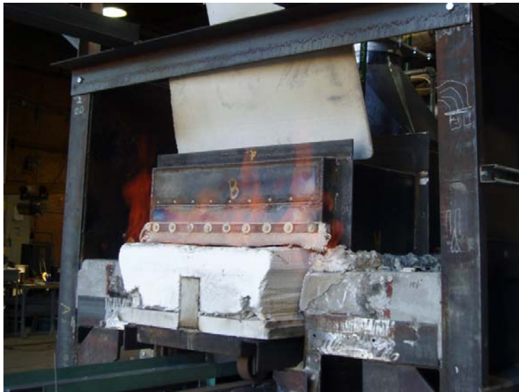
Figure 2-7-6(b). Flame shooting out from the discharge end of LHF when a sample tray was in Zone 3.
