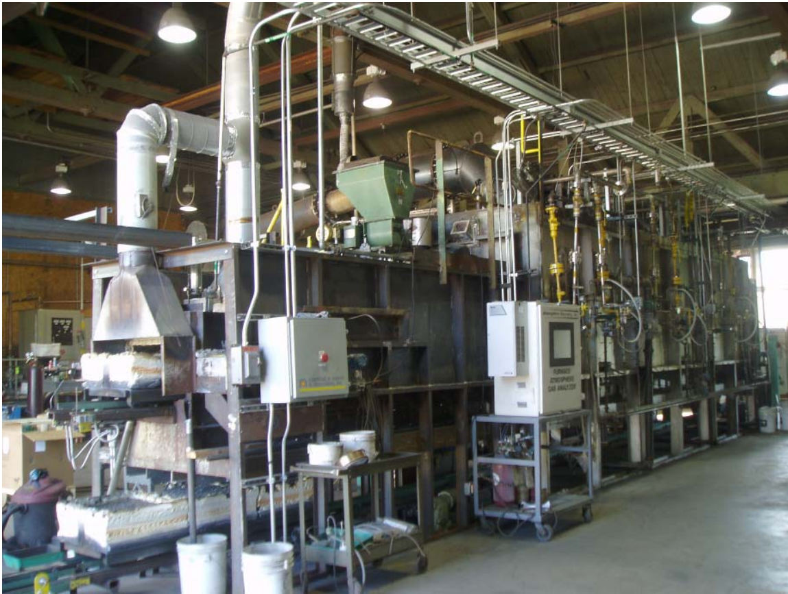
Figure 2-3-3. General view of the three hot zones and the cooling zone of LHF with oxy-fuel burners.
