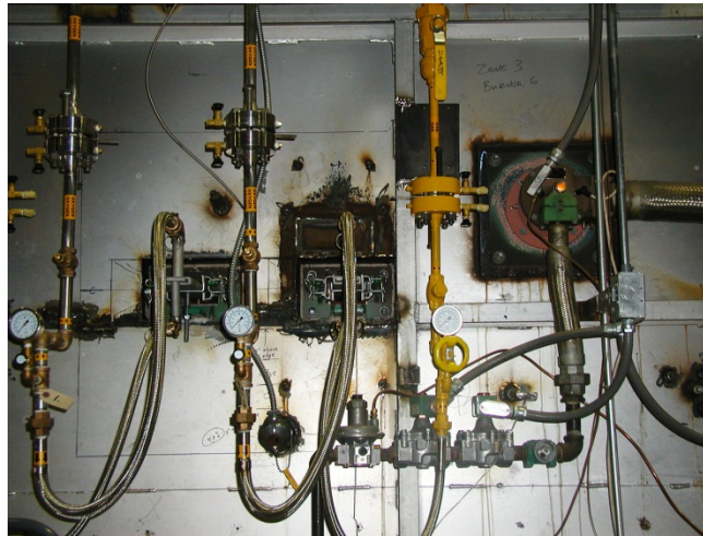
Figure 4-12. Dual – Combustion System Burner Arrangement
