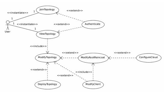
Figure 3. High level use case diagram for the Raincoat application.
