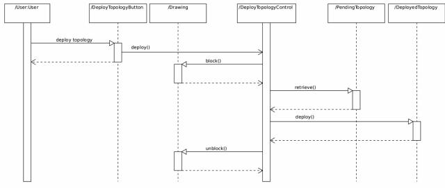
Figure 6. Sequence Diagram for the DeployTopology use case.
