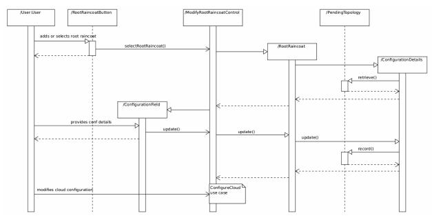
Figure 7. Sequence Diagram for the ModifyRootRaincoat use case.
