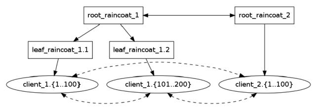
**Figure 1.** The purpose of leaf and root Raincoats in a topology supporting 300 clients total. Solid lines represent VPN providers and dotted lines represent overlay network connectivity.
