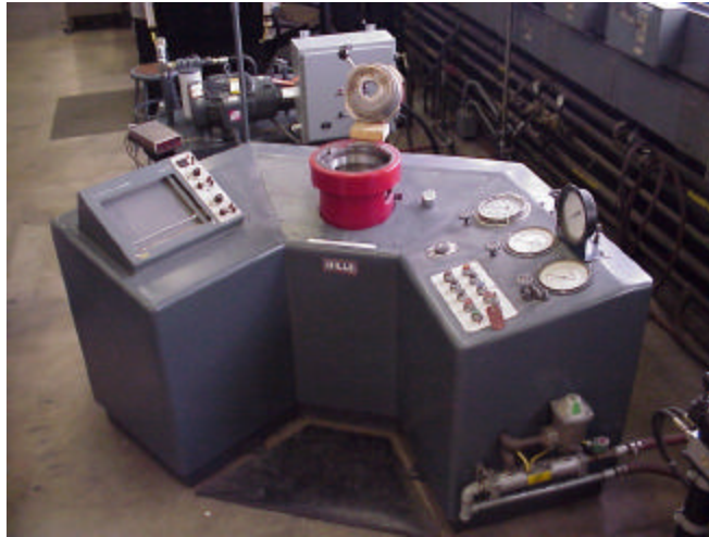
Figure 6.1: Photograph of the Hille-Wallace hydraulic press used for conducting the sheared edge stretching tests
