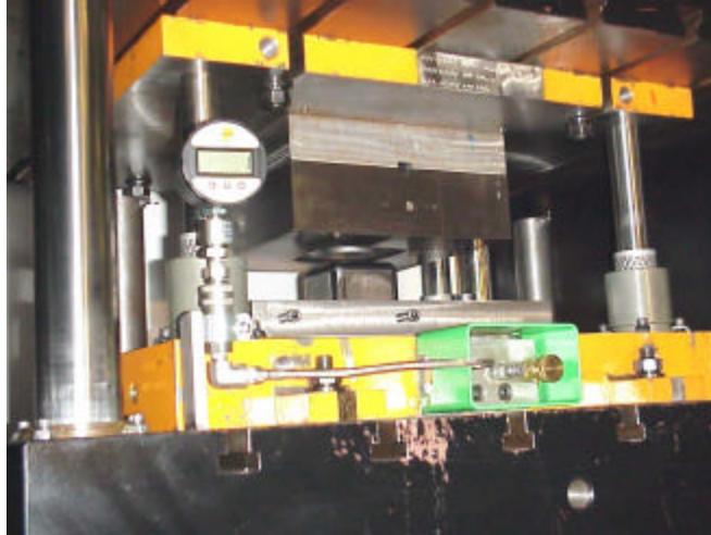
Figure 10.2: Square Draw tooling as installed in the servohydraulic press
