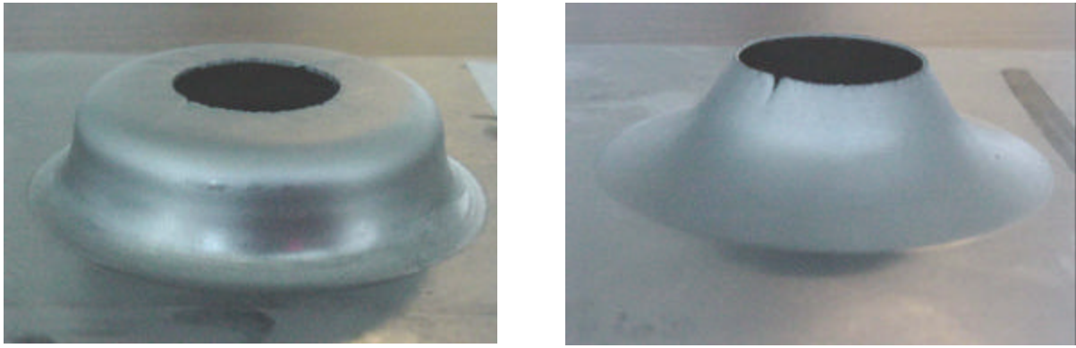
Figure 6.2: Geometries of the hole expansion and hole extrusion test specimens
