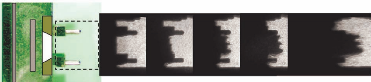
Figure 3.4. Experimental data from a shadowgraphy experiment. Shown are five frames, each with ~2ns exposure, timed ~15 ns apart. Clearly evident is an expanding aluminum plasma.
