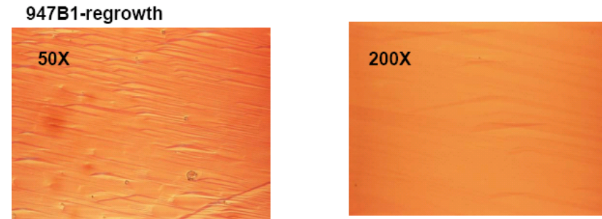
Figure 24: Optical Nomarski microscope image of the heteroepitaxial undoped GaN on m -plane bulk substrate. (left) 50x objective, (right) 200x objective. Very smooth surfaces are revealed on both length scales.
