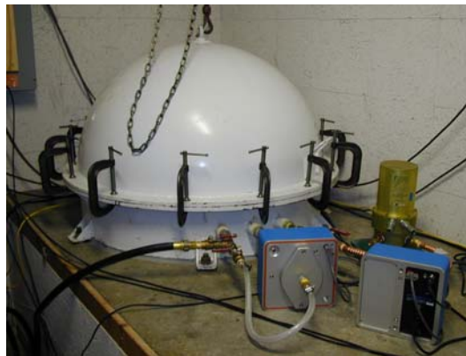
Figure 3.4.2 Sensor testing chamber, acoustic piston-phone and acoustic reference sensor (MB2000 – SN1380).
