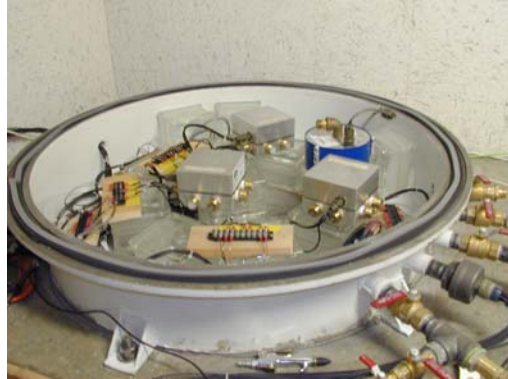
Figure 3.4.1 Infrasound sensor configuration for sensor testing in FACT site acoustic chamber.
