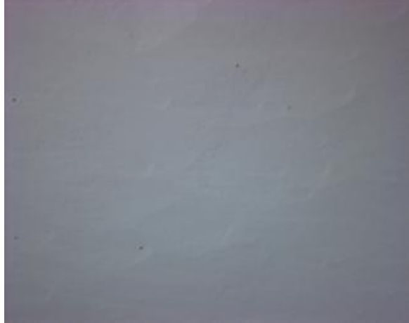
Figure 5: Nomarski DIC image, taken at 50x, of 6 \mu\text{m} of AlGaIn overgrowth
