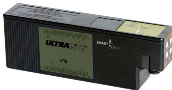
Figure 30. A picture of the LI-145 lithium ion battery from UltraLife, for U.S. military soldier power.
