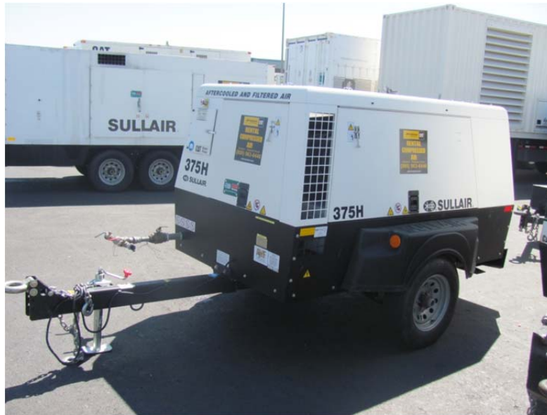
Figure 13. Diesel powered portable air compressor (Sullair 375H AF) at Peterson Power, San Leandro, CA.
