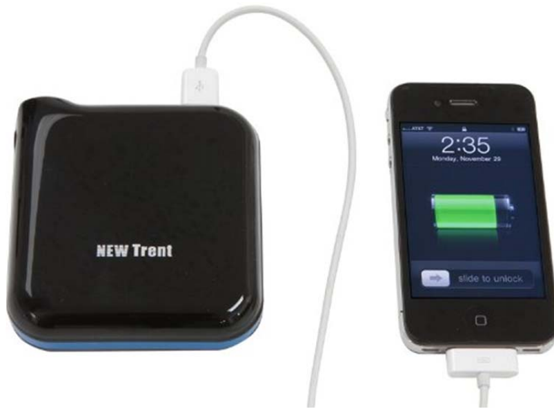
Figure 34. The New Trent iCruiser IMP1000 (on the left) recharging an iPhone 4. It has an 11,000 mAh lithium polymer battery. Specifications are given in Table 24.
