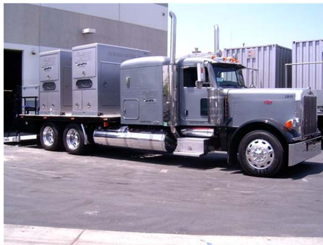
Figure 21. Live broadcast truck with two 175KW-1400A Movie Quiet generators permanently mounted. Photo courtesy of Saunders Electric.
