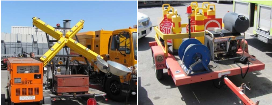
Figure 16. Pictures of an aviation light cross (left), and light ropes with a portable generator (right) in use at SFO.
