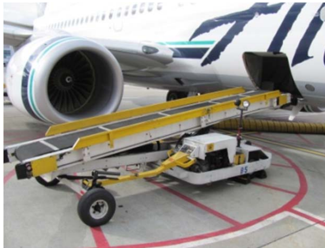
Figure 14. Example of a luggage belt loader in use at SFO.
