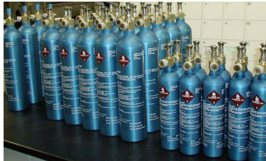
ECD, Inc. – Portable Metal Hydride Canisters
