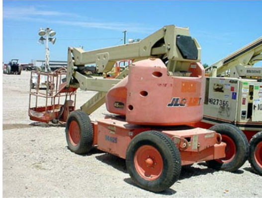
Figure 17. Photograph of a boom lift being used at SFO.
