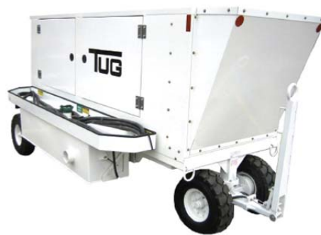
Figure 15. TUG GP400-120 120 kVA ground power unit.
