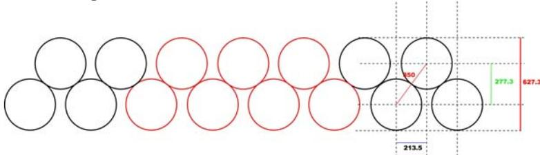
**Figure 16** Arrangement of scintillating fibers in a tracker station plane as used in the MICE trackers). The fiber diameter is 350  $\mu\text{m}$ , 7 fibers/channel, 1.63 mm/chan, which gives a resolution of 0.47 mm per plane. The fibers amount to 0.45%  $X_0$  per double plane.
