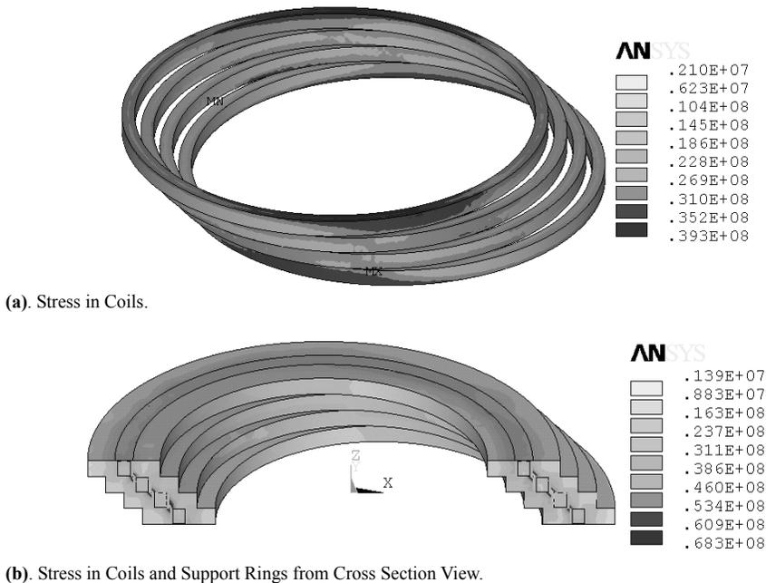
FIGURE 5. Stress Distribution (Value in Pascal) at the Peak Current 14 kA.
