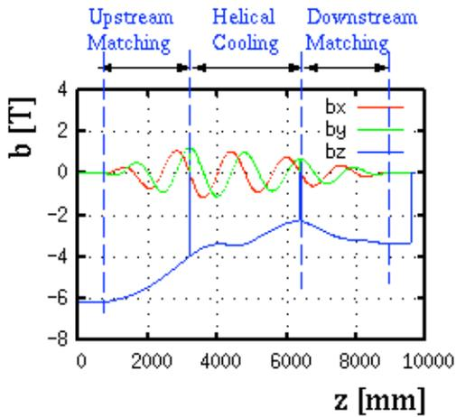
Figure 2: Magnetic field of reference particle in MANX
