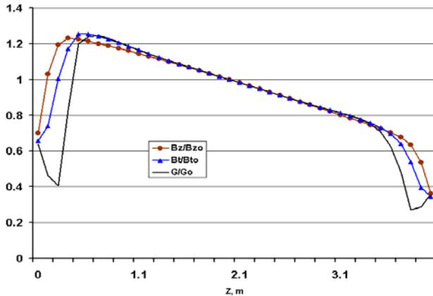
Figure 2: Field distribution related to the values at  $z=2$  m ( $B_{z0}=-3.37$  T,  $B_{t0}=1.04$  T,  $G_0=-0.9$  T/m).
