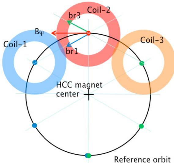
Figure 3: Schematic view of the HS coil from the end of HCC.
