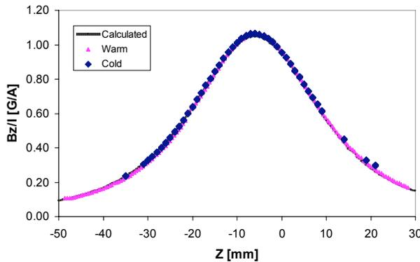
Figure 4: Longitudinal Field on axis vs. Calculation
