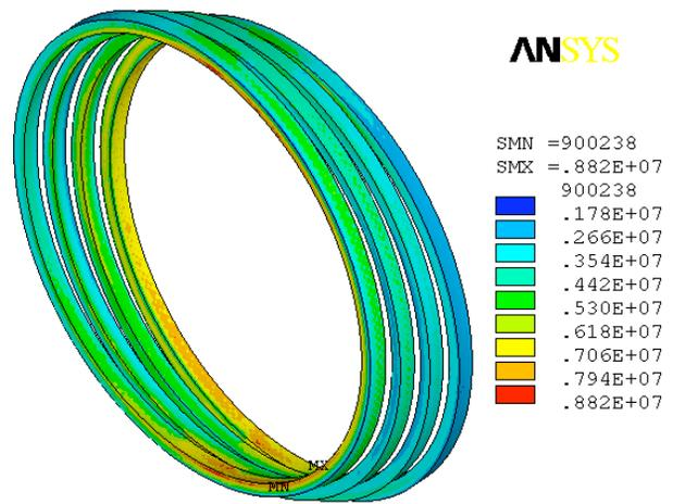
Figure 2: Coils stress at the peak current 14 kA.
