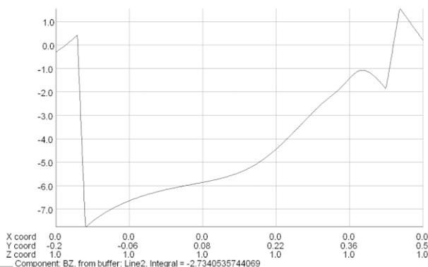
Figure 8: Helical Solenoid with triangular coils. Bz field distribution from radius -0.2 m to 0.5 m.
