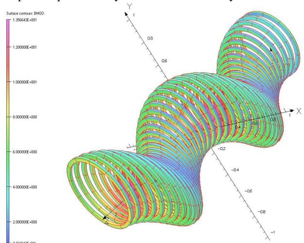
Figure 1: Helical Solenoid geometry and flux density.
