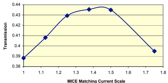
Figure 4: Muon transmission in the HCC channel as a function of the MICE matching coil current. The current is shown as a scale factor to be applied to the nominal MICE matching coil current.
