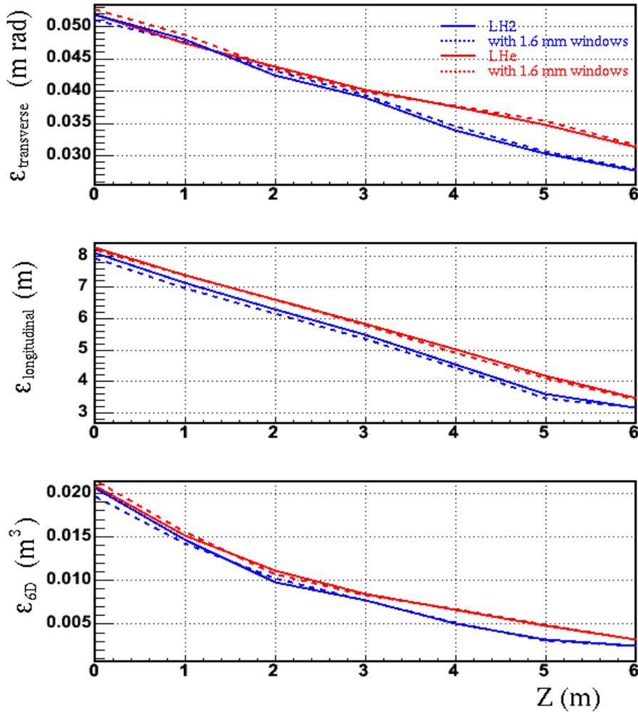
**Figure 4** Simulations showing normalized emittance evolution for particles that survive to 6 m for a HCC pre-cooler filled with liquid hydrogen (blue) or liquid helium (red), with (dashed) and without (solid) 1.6 mm thick aluminum windows on each end.
