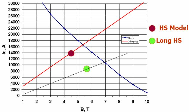
FIGURE 1. Cable  $I_c(B)$  Dependence and Load Lines for Long HS and for HS Four-Coil Model.
