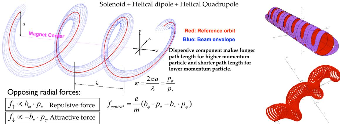
**FIGURE 1.** (left) Helical-channel principle; (top-right) conventional “Siberian snake” solution with individual windings providing the required solenoidal, helical dipole, and helical quadrupole fields; (bottom-right) Helical Solenoid implementation with the same acceptance and the three required fields produced using simple offset coils only half the diameter of the conventional magnet.
