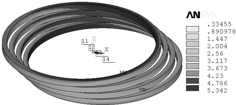
FIGURE 2. Four-Coil Geometry and Magnetic Flux Density Distribution (Values in T) at 14 kA.
