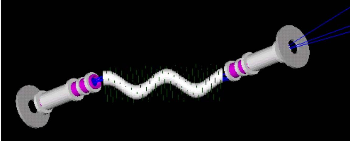
Figure 9 *A G4beamline representation of the off-axis matching configuration where the HCC is placed at a  $45^\circ$  orientation to the MICE spectrometer so that the beam is oriented along the reference path at entrance into the HCC.*
