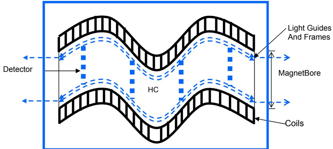
**Figure 17** *Schematic of placement of four tracker stations inside of HCC. There are also tracker stations upstream and downstream of the HCC, which are not shown. Detector planes outside of the magnet are not shown.*
