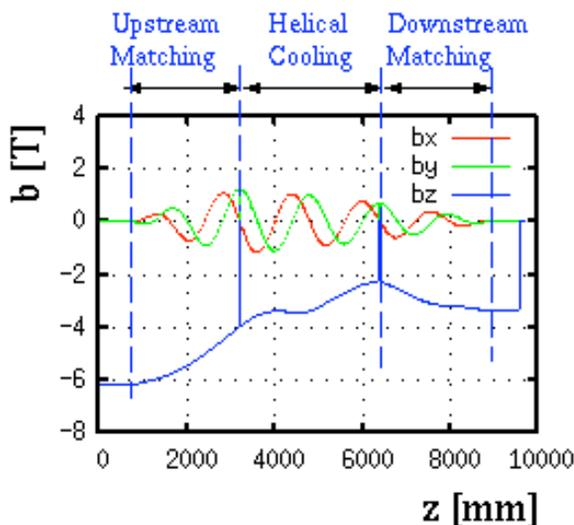
Figure 3: Field strength along the reference orbit in the MANX channel.
