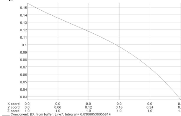
Figure 6: Helical Quadrupole transverse field Bt.
