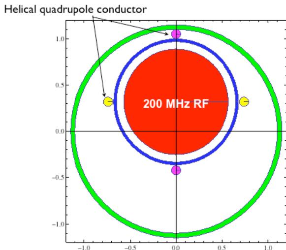
Figure 5: Schematic view of a new HS configuration with a helical quadrupole conductor.
