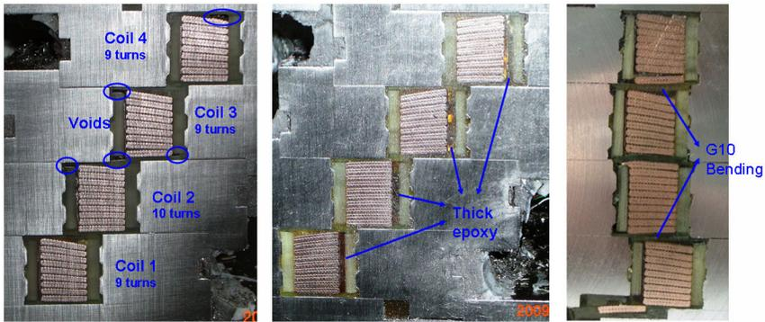
FIGURE 10. Post-Test Autopsy and Inspection.
