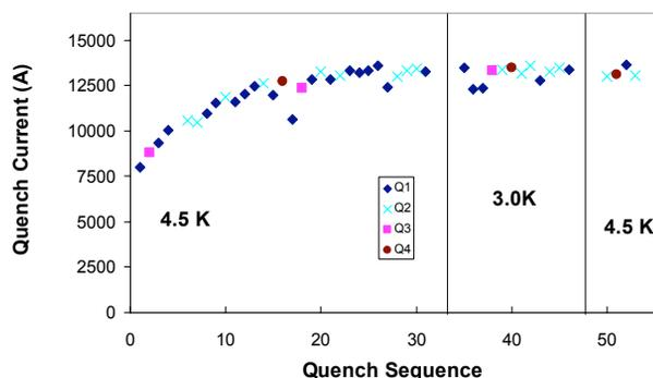
Figure 3: Quench Performance of HSM01. Coils are designation Q1-Q4 with Q1 closest to the positive lead.
