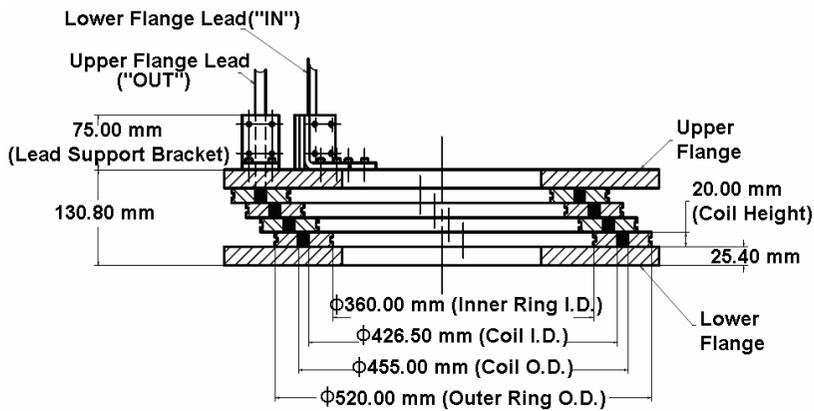
FIGURE 3. The Model Design Sketch in Cross Section View.
