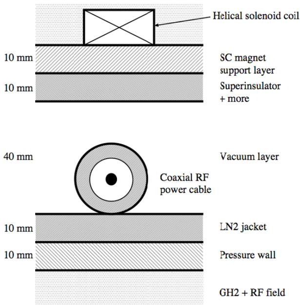
Figure 2: Schematic draw of layers between the HS coil and the high pressurizing hydrogen filled RF cavity.
