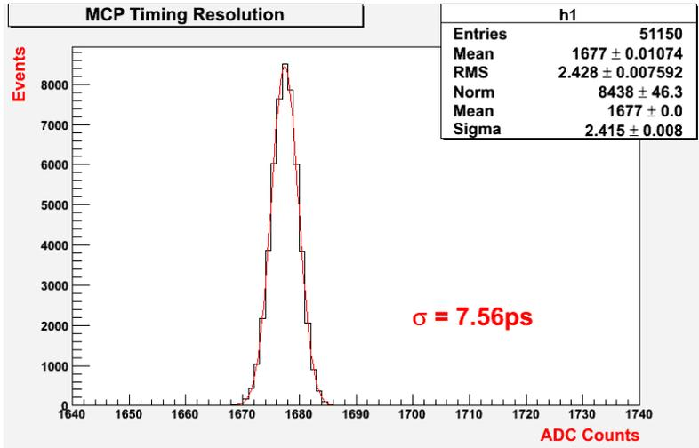
Figure 14 Measurement of the time difference between two commercial MCPs with 25 $\mu\text{m}$  pores. Data are for a 408nm laser with ~50 photoelectrons, at the laser test stand at Argonne (Hamamatsu PLP-10 picosecond laser and a commercial CAMAC readout electronics system). The intrinsic jitter of the system is ~4ps and it has a resolution of 3.13ps [22]. The individual MCPs therefore have an intrinsic resolution about 4 ps.
