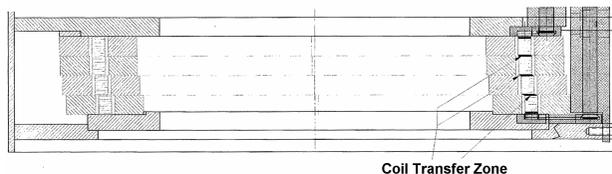
FIGURE 7. Cross Section of the Transition Turns.
