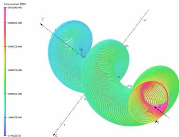
Figure 1: Helical Solenoid geometry and flux density.
