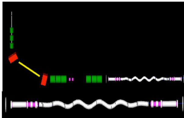
Figure 1: MANX baseline matching design. (a) MANX layout including beam line. (b) Enlarged MANX HCC with baseline matching sections.
