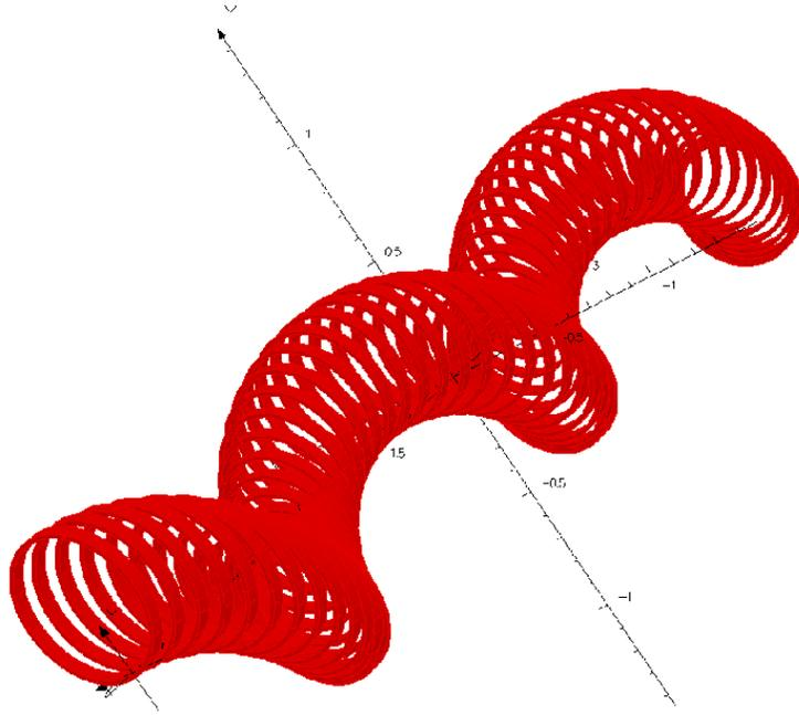
**Figure 5** Conceptual picture of a HCC segment using the helical solenoid, which provides solenoid, helical dipole, and helical quadrupole fields. Although at first glance it looks like a child’s “slinky” toy, the coils are independent rings. For the MANX simulation shown in the next figures below, each ring diameter is 0.5 m and ~60 coils are used for the 3.2 m long HCC.
