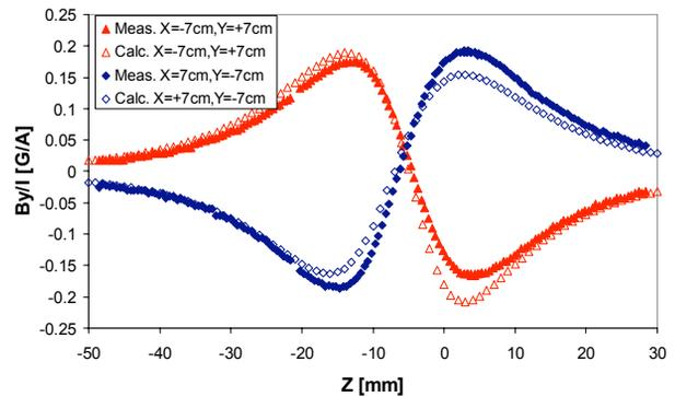
Figure 5: Representative Transverse Field/Current vs. Calculation
