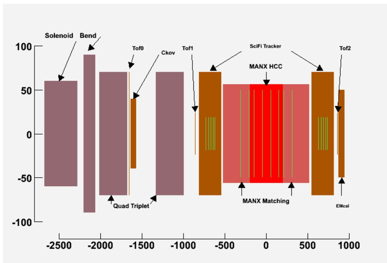
**Figure 11** Sketch of RAL MICE muon beam line elements (violet) with MANX LHe-filled helical cooling channel (red) and evacuated matching sections (salmon) positioned between MICE spectrometers (brown). The decay solenoid is at the left. The dimensions are in cm.
