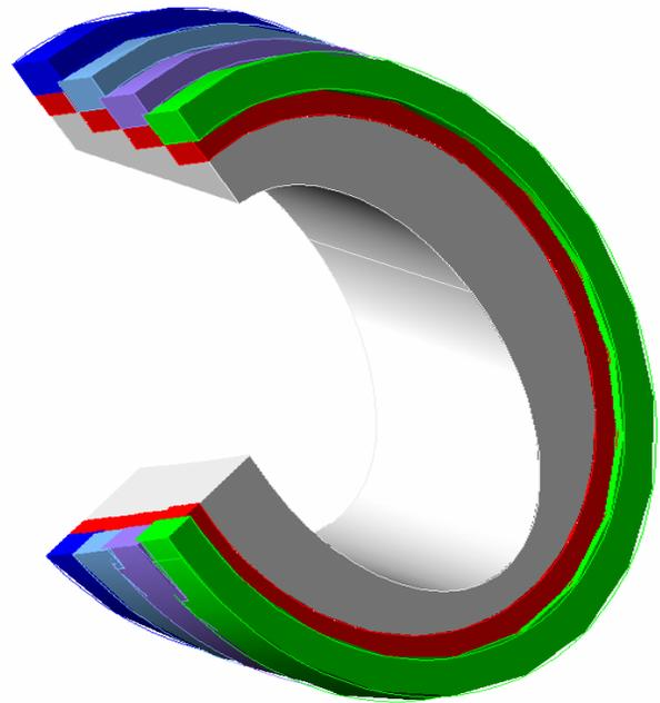
Figure 4: Helical Solenoid short section geometry. Inner support (grey), superconducting coil (red) and outer collar rings (green-blue).
