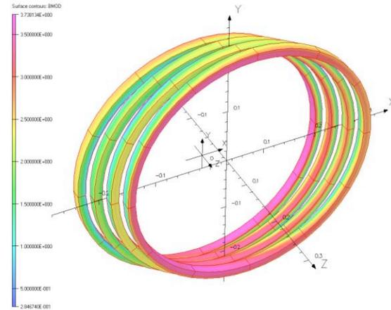
Figure 1: 4-Coil geometry and flux density.
