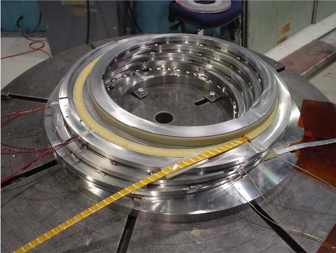
**Figure 28** *Assembly of 4-coil model before 4<sup>th</sup> coil has been wound*
