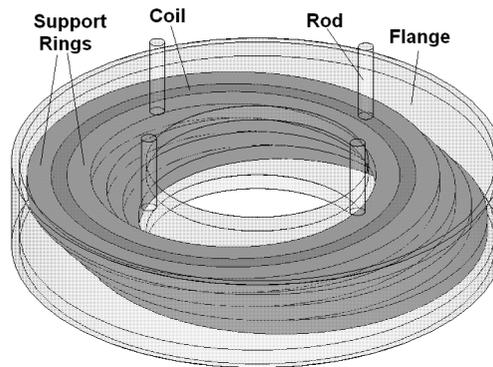
FIGURE 4. 3D Mechanical Model in ANSYS.
