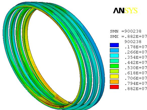
Figure 26 Coil stress at peak current of 14 kiloAmp
