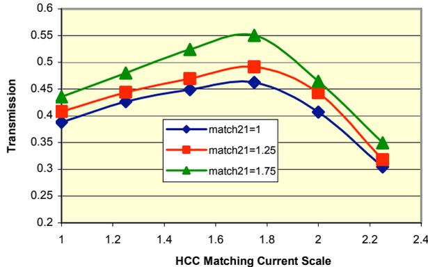
Figure 5: Muon transmission in the HCC channel as a function of the current in the first two HCC short solenoids. The current is shown as a scale factor to be applied to the nominal current in those solenoids. The different curves shown correspond to different currents in the MICE matching coils.
