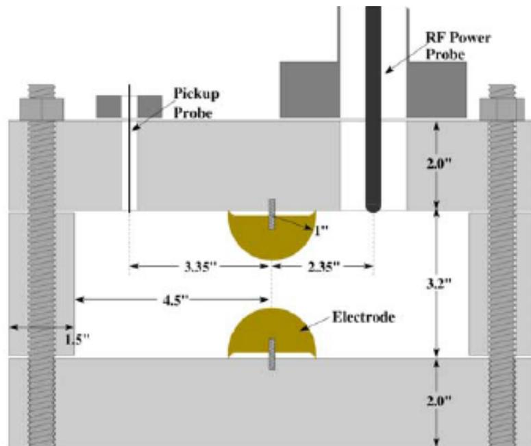
**Figure 23 High Pressure Gas-filled RF Test Cell**
