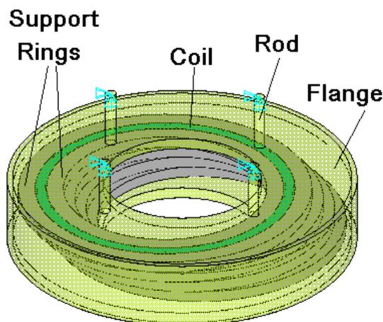
Figure 1: HSM01 Coil Layout
