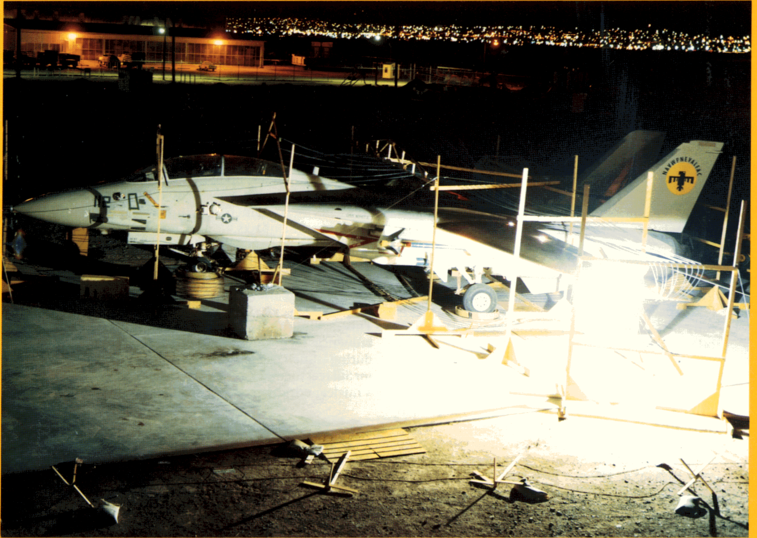
A Navy F-14A is subjected to a dramatic night test at the Sandia Lightning Simulator Facility. The test series was designed to determine how a lightning strike affects the sensitive computer electronics on this aircraft. The 80,000-amp charge entered through the nose and exited via the wing tip (the bright flash). The spark lasted for one second and was the sole light source for the picture.
