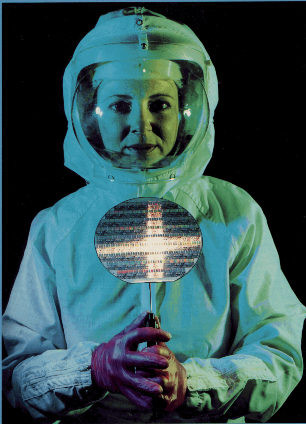
Sandia researcher April Howard displays a wafer of semiconductor chips manufactured in Sandia's Microelectronics Development Laboratory. The lab incorporates a 13,000-ft 2 clean room that uses the laminar air flow clean room principle invented at Sandia to make prototype semiconductor chips for weapons, satellites, and spacecraft.
