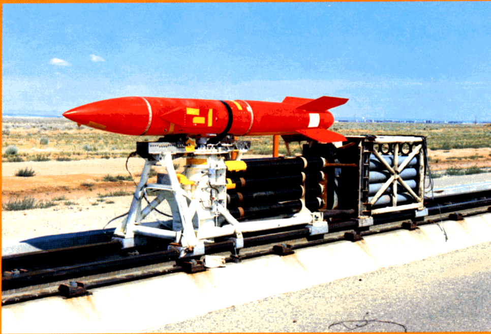
MK/B 61 shape on rocket sled for parachute system test. The rocket sled facility can also be used to study severe transportation accidents of nuclear material shipping containers.
