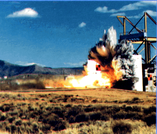
An F-4 Phantom slams head-on into concrete barrier at 480 miles per hour in test at Sandia's rocket-sled facility south of Albuquerque. The work is expected to advance the state of the art in designing large structures for nuclear power plants.
