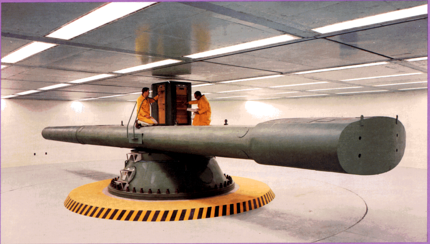
The largest centrifuge in the free world (8.8-m [29-ft] radius) is in the Sandia Centrifuge Facility in Albuquerque, NM.
