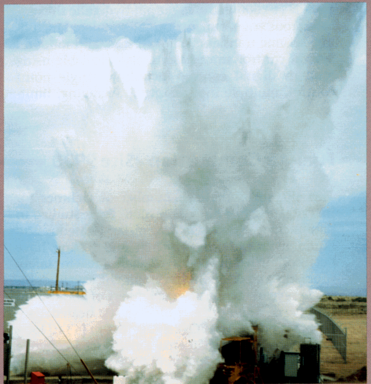
Large-scale steam explosion created by molten fuel-coolant interaction at Sandia's Albuquerque location (Site 9940).
