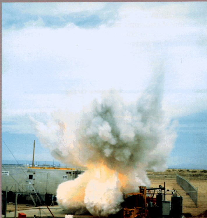
Large-scale steam explosion created by molten fuel-coolant interaction at Sandia's Albuquerque location (Site 9940).
