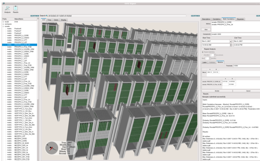
Figure 13: Actual rendering of the Red Storm platform zoomed in on the partition on which data were taken. The nodes are colored red if below the user-defined probabilistic threshold for being too unreliable and green otherwise. Grey indicates there was no data in the display time window for that resource for the metric being displayed.
