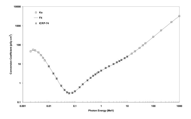
Fig. 5. Kerma conversion coefficients for 0.007 cm, 0.3 cm, and 1 cm depths in the slab phantom in units of pGy cm<sup>2</sup> and the fits determined using the values in Table 2 according to Equation 1. Also shown are the values of effective dose using the phantoms of ICRP-110 and the methodology described in ICRP-103.
