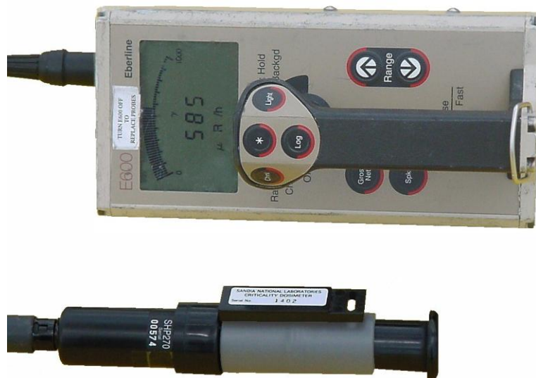
Figure 2: The SNL “PNAD Quick-Scan” process an SHP270 probe (shield in closed position) connected to an Eberline E600. The SHP270 probe is calibrated to 137Cs.
