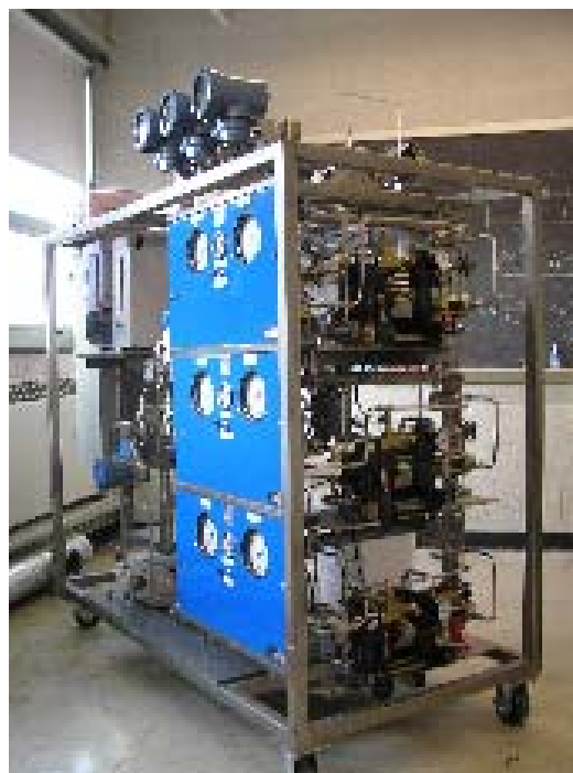
Figure 7.1: (a) Multi-channel microreactor plate (b) Compact Skid-mounted Micro-reactor-based Distributed Production Plant (1 – 10 kg/h)
