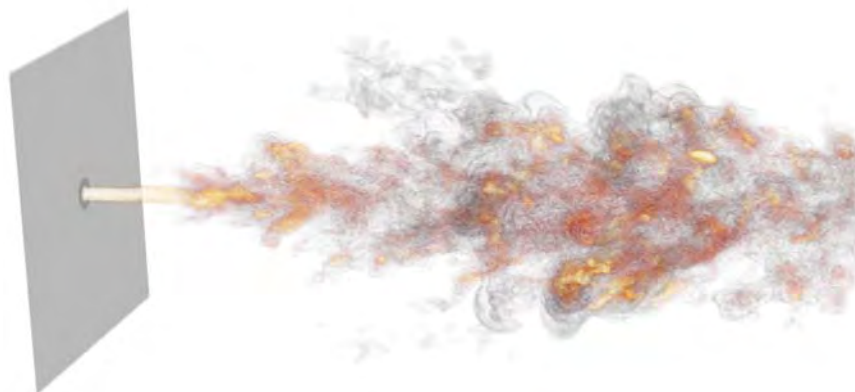
Figure 14. Volume rendering of the number density of the small particles.
