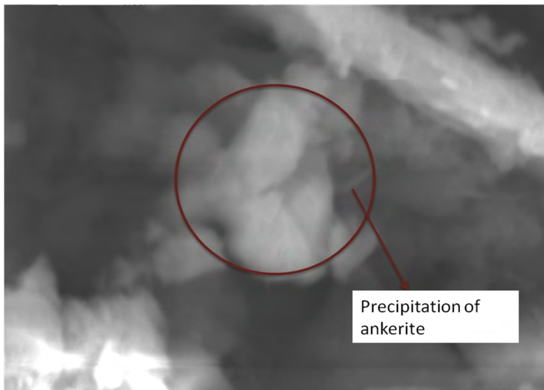
Figure 6d: SEM image of Ankerite growth in the final sample
