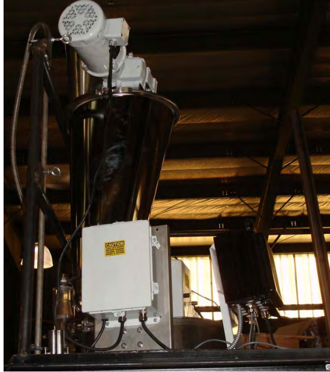
Figure 19. K-Tron loss-in-weight twin-screw coal feeder applied in oxy-coal combustion lab, University of Utah
