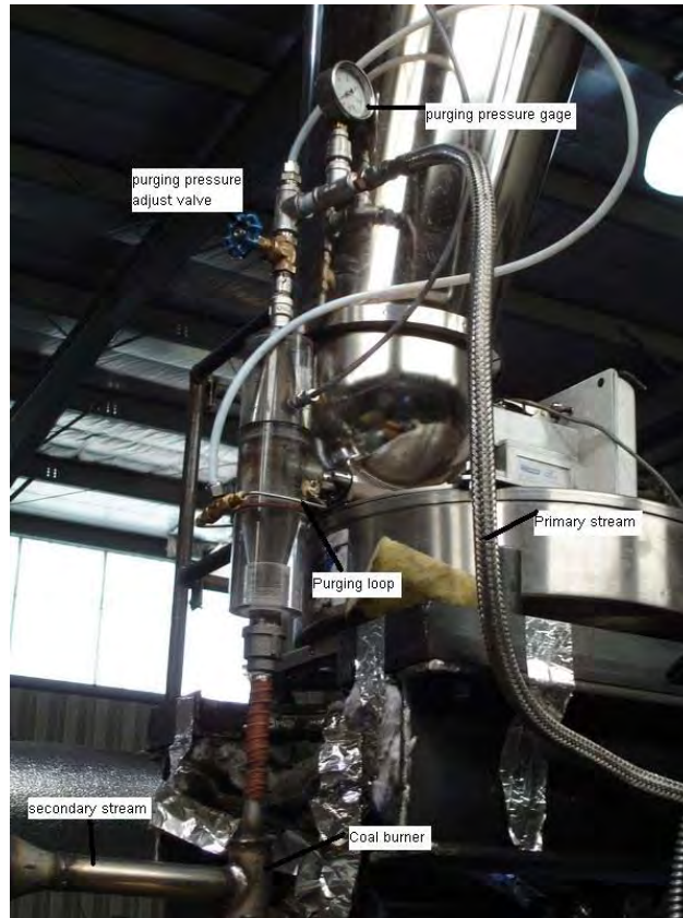
Figure 20. An eductor design schematic in oxy-coal combustion lab, University of Utah
