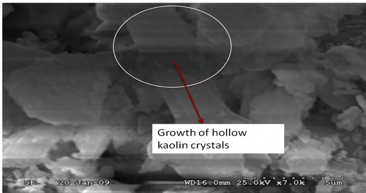
Figure 17: Growth of hollow kaolin crystals
