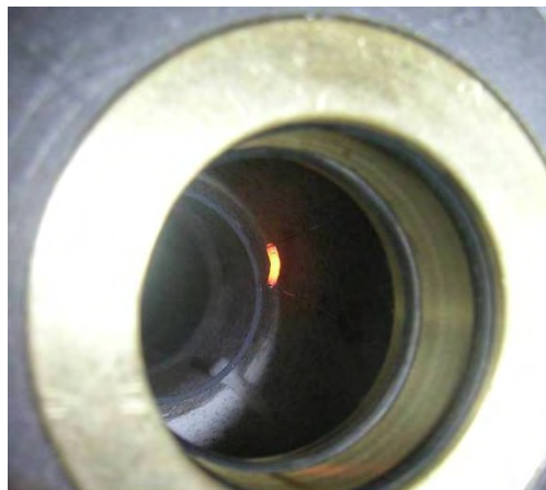
Figure 2. Glow plug ignition system and brass insert in vessel cap.
