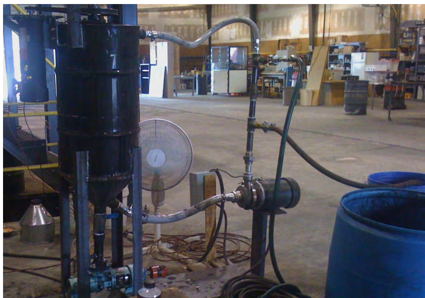
Figure 67. Prototype coal slurry feed system. The progressive cavity pump body is seen below the tank, the motor for the mixer is vertically mounted in the upper-left corner of the photo. The recirculation pump is near the center of the photo.
