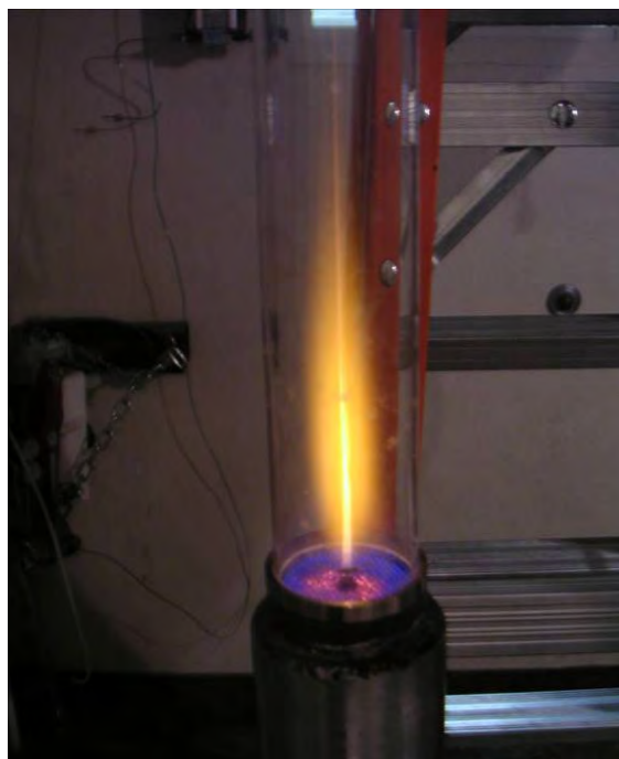
Figure 4. Atmospheric demonstration of coal feeding through burner with glowing surface.
