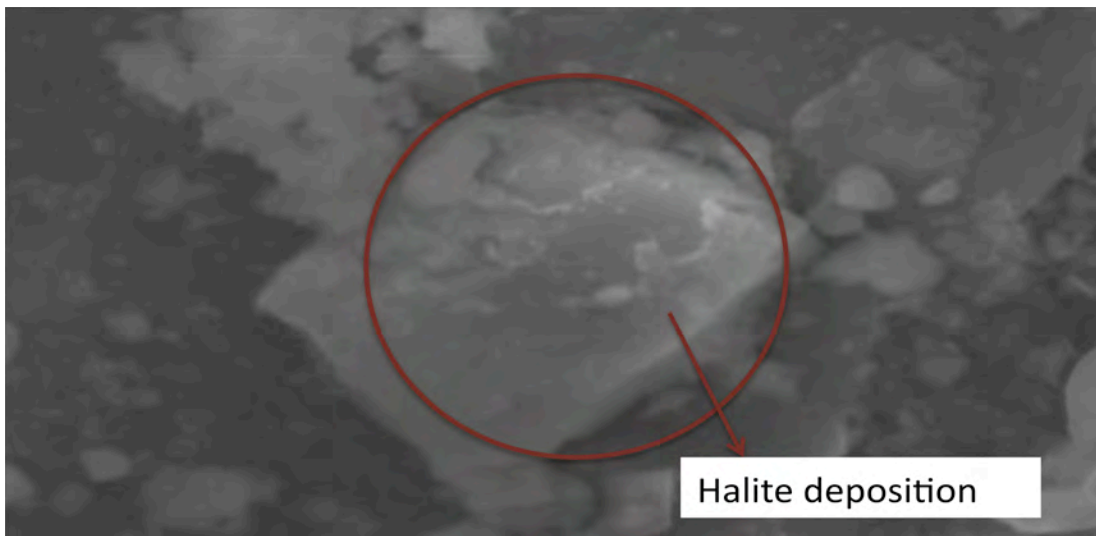
Figure 6c: SEM image at 3kx magnification showing deposition of Halite chunks
