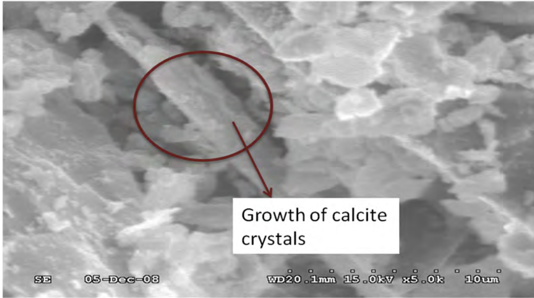
Figure 8a: Calcite crystals growing in interstitial spaces between plagioclase feldspar
