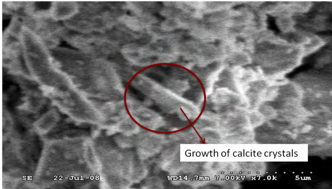
Figure 7c: SEM image showing the growth of calcite after 134 days indicative of mineral precipitation reactions
