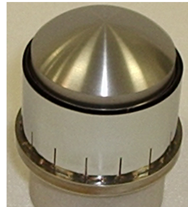
Figure 8. Dome cathode for beam analyzer experiment
