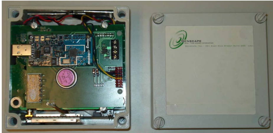
Figure 4-9: Form factor design for the new transmission line monitor
