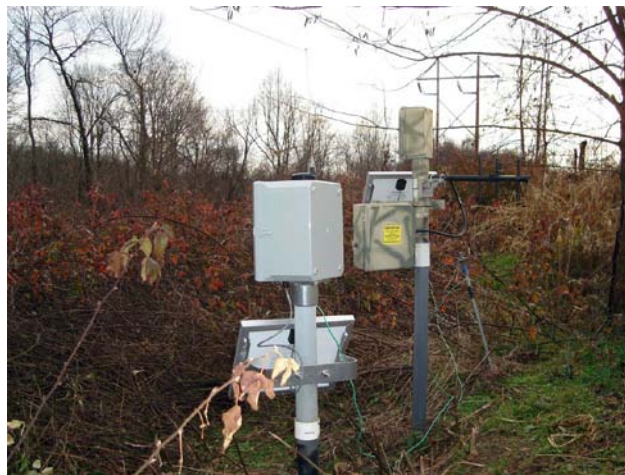
Figure 5-2: Side-by-side deployment of existing transmission line monitor (right) and a prototype Mote-based transmission line prototype (left) at a power line field test site.
