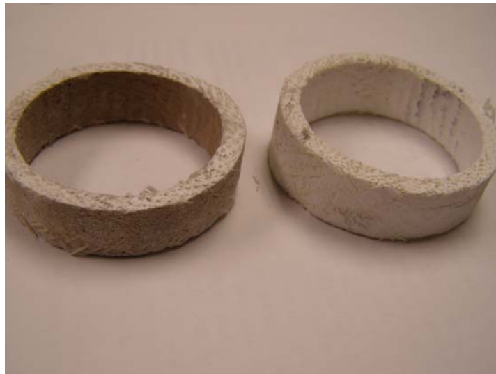
Figure 12: Photo of the rings of the new (right) and used (left) filter
