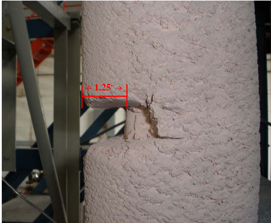
Figure 23: Pictures of the filter loaded with flyash after being subjected to an air/flyash/steam mixture for nearly 130 hours.
