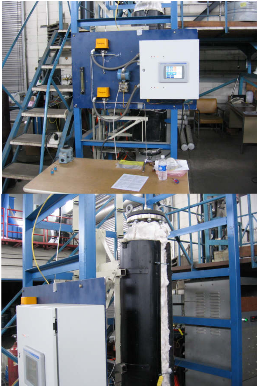
Figure 4: (top) Controller box, differential pressure meter and solenoid valves; (bottom) Reactor and furnace
