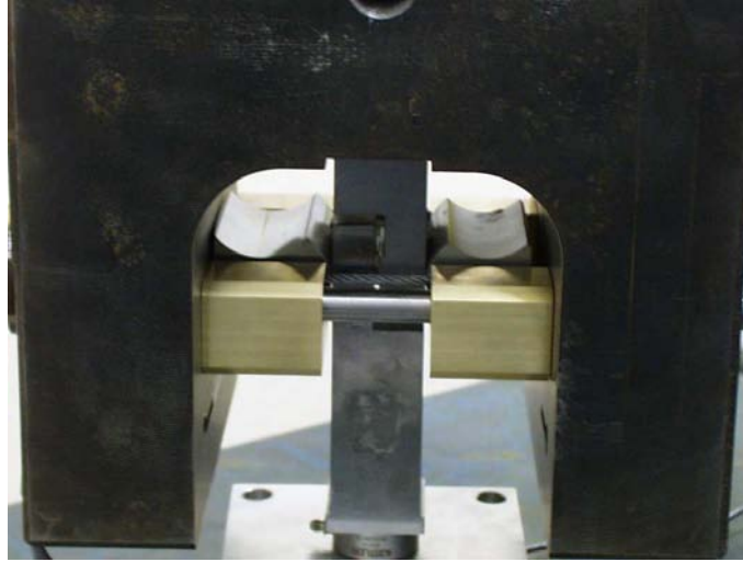
Figure 4.14. Assembly Fixture for Rollers.
