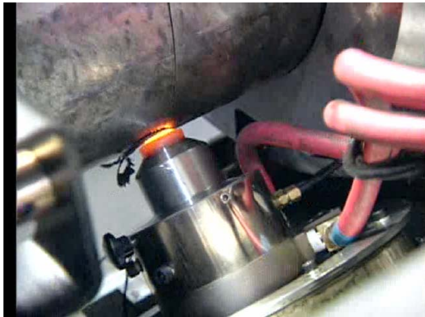
Fig. 3: A prototype FSW system for steel piping welding, developed by MegaStir
