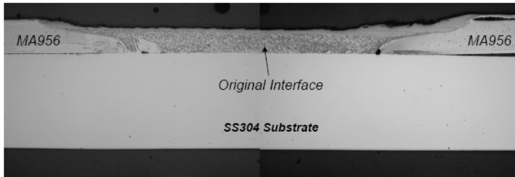
Fig. 6: Cross-section view of the butt weld. SS304 substrate is also shown underneath the weld.
