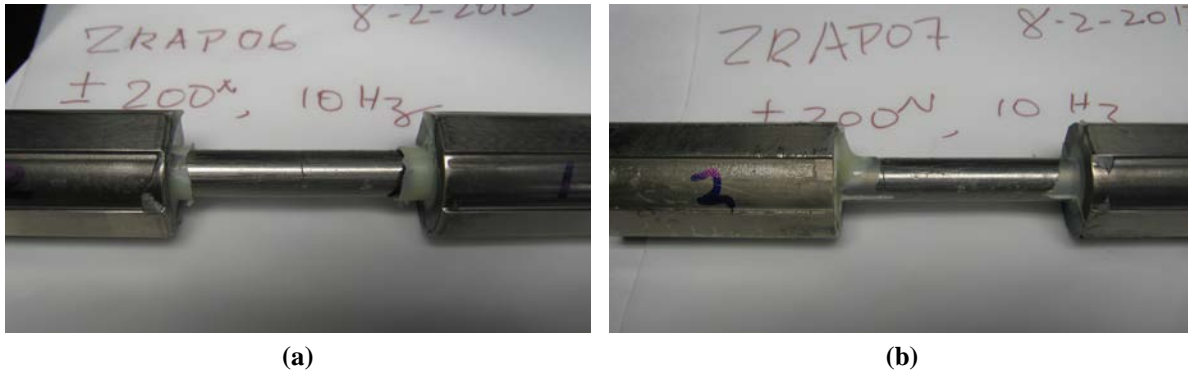
Fig. 20. Images showing the fractured rods of (a) ZRAP06 and (b) ZRAP07.
