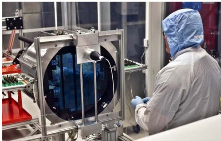
Figure 7. The Micro-Epsilon confocal chromatic displacement system being used to perform a quick scan of the CCD array after arrival at the Blanco telescope. The simple rail system was built to allow quick inspection of a CCD surface relative to its immediate neighbors. The same instrument, mounted on a precision stage system, is separately used to survey the focal plane array through the flat vessel window. Photo credit T. Abbott (CTIO).
