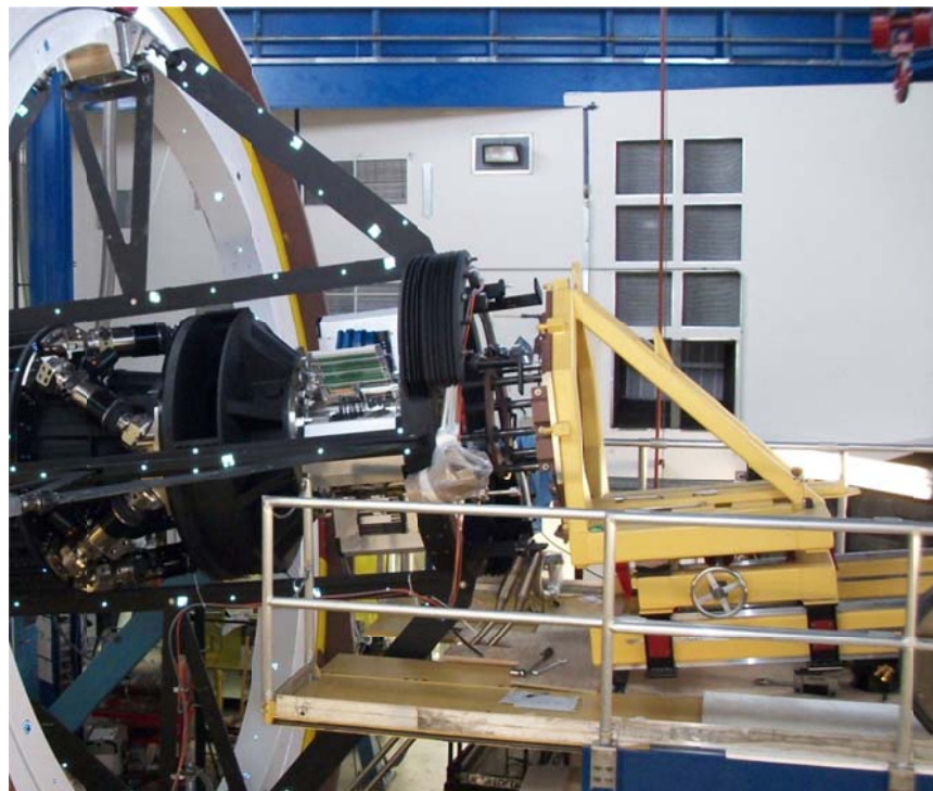
Figure 10. Imager installation testing on the Telescope Simulator. The imager has been translated forward and mated to the back of the corrector.
