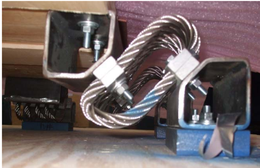
Figure 5. Isolation coils after arrival in Chile. View along listing edge of the suspension system with the imager not yet removed from crate. Crate floor shows some sign of coil contact even with the additional spacer shown under the coil mounting bracket.
