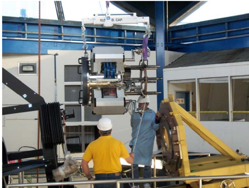
Figure 9. Imager installation testing on the Telescope Simulator. The crane is being used to transfer the imager onto its installation fixture. The fixture supports the cantilevered imager and permits adjustment of its transverse & vertical position and its pitch & roll angles as it moves axially into the prime focus cage where it mates it with the corrector.
