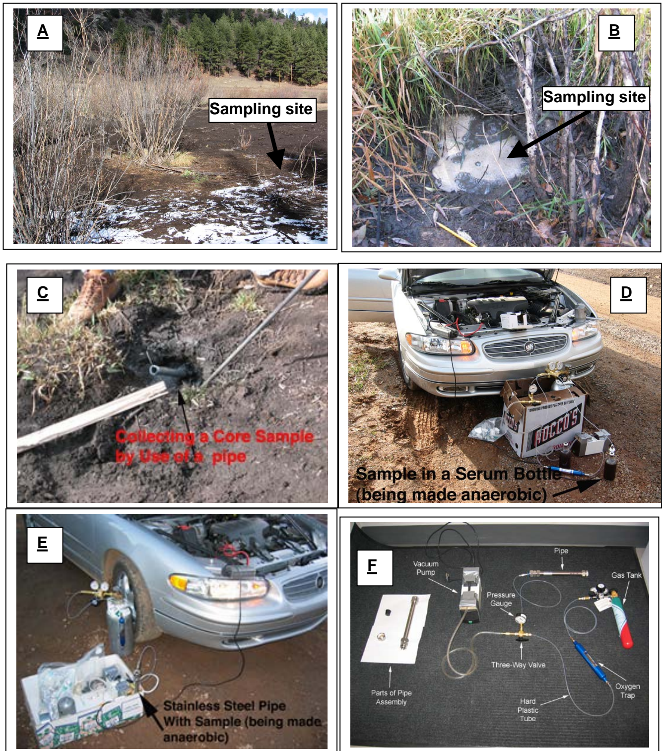
Figure 5. (a) BP-Amoco Texas Creek methane seep site (b), active methane seep and sample collection site, (c) soil core collection with pipe (d) serum bottle being made anaerobic, (e) soil samples in pipe being made anaerobic, and (f) detailed view of anaerobic sampling system.
