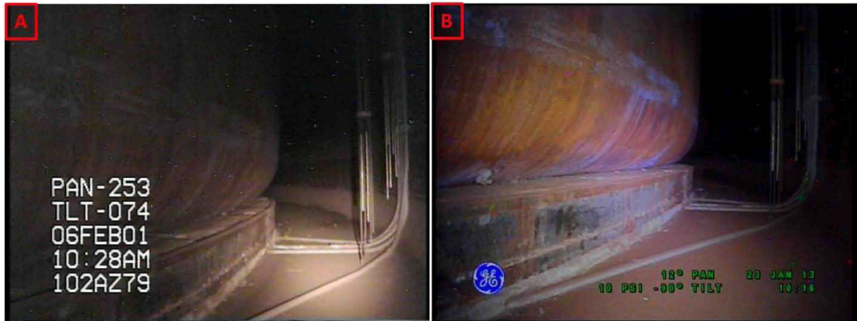
Figure 3-8. Riser 79 Lower Knuckle and Annulus Floor Comparisons Between Inspections on February 6, 2001 (A) and January 23, 2013 (B) Looking Towards Riser 99
