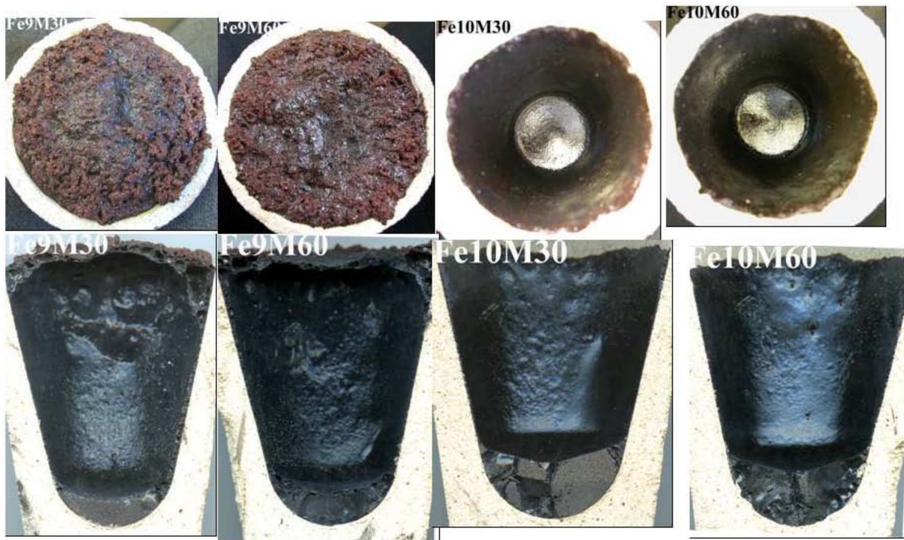
Figure 2.1. Top and cross section views of high iron feed samples after VGF experiments: i) HLW-NG-Fe9; j) HLW-NG-Fe10.
