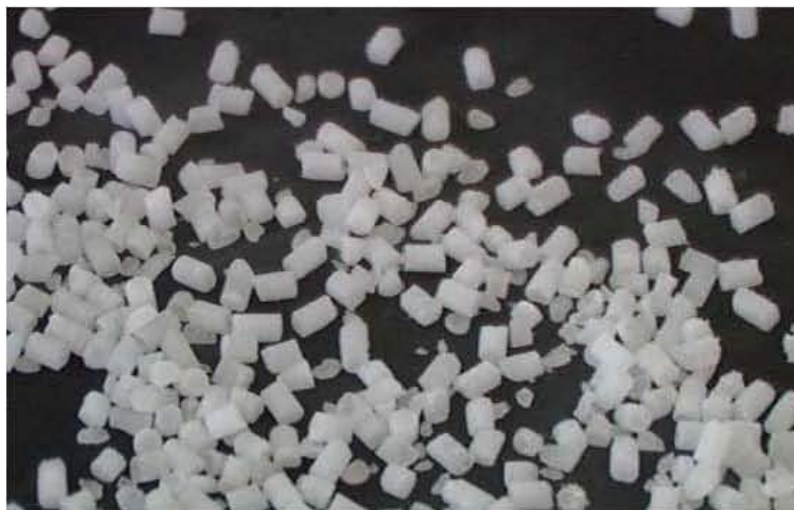
Figure 2-9. Typical CO2 Blasting Pellets
