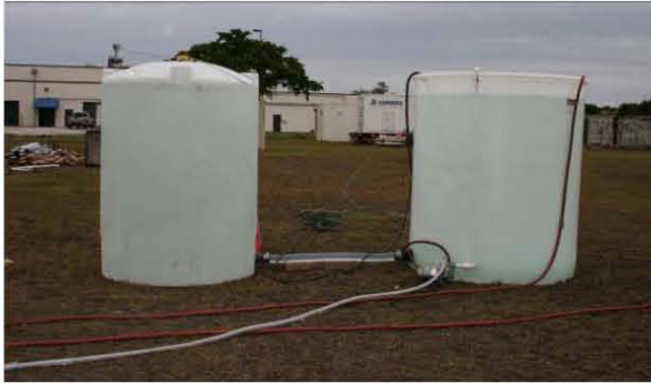
Figure 22. 1000-gallon and 1500-gallon water tanks.
