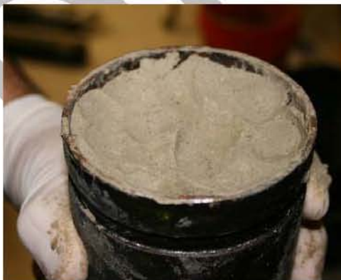
Figure 18. Close up of a Bentonite plug.
