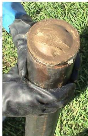
Figure 21. 4-ft Kmag plug.
