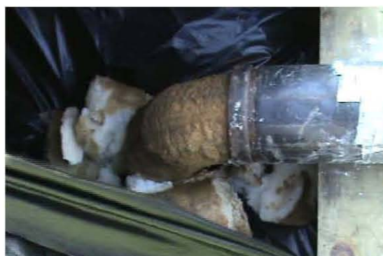
Figure 17. Phosphate plug during extrusion test.
