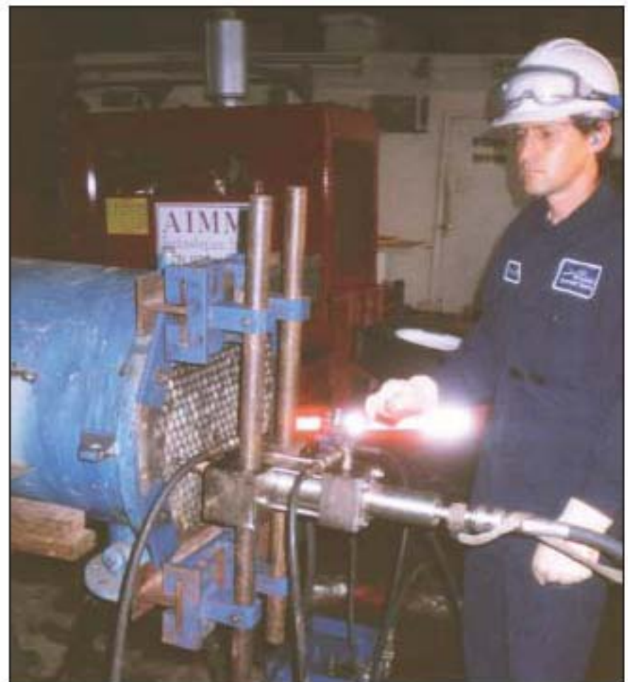
AIMM employee Americo Almeida operates a Hydrokinetic ram assembly. Hydrokinetics is a new tube cleaning technology developed by AIMM, based in LaMarque, Texas.
