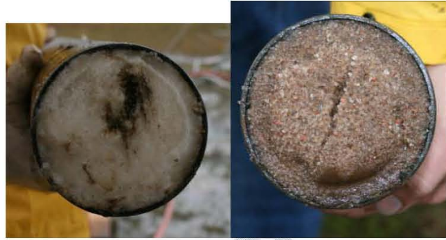
Figure 34. 4 ft Na-Al-Si plug (left) and Kmag plug (right) after unplugging trials with AIMM.
