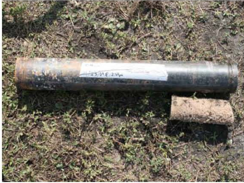
Figure 29. 6 in of Kmag unplugged from 2 ft blockage section.
