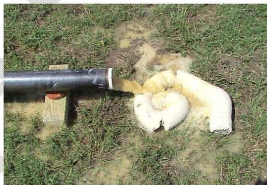
Figure 15. 4ft Kaolin 66% after extrusion test.
