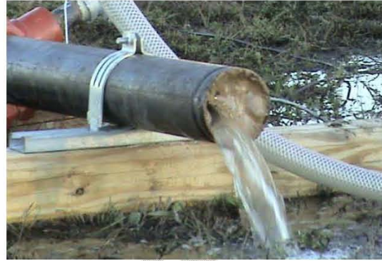
Figure 30. Flow achieved through 2 ft Kmag plug.
