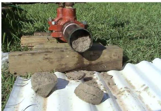
Figure 14. Kmag plug falling off during extrusion test.
