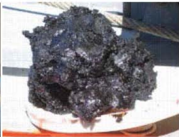
Figure 6-5. Pipeline Blockage or Foulants Handled by the Hydrokinetics System
