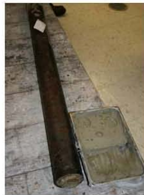
Figure 19. 4 ft Bentonite plug.
