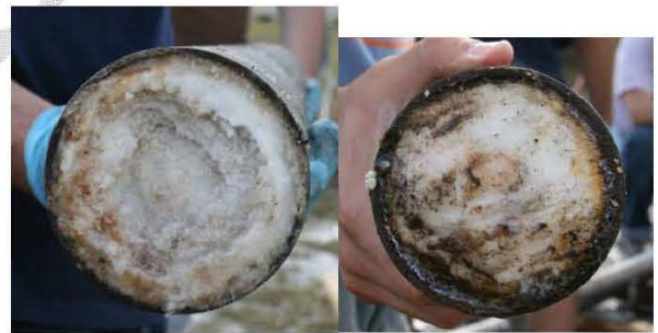
Figure 32. 4 ft Na-Al-Si plug after unplugging trials with AIMM. Front side (left) and back side (right).
