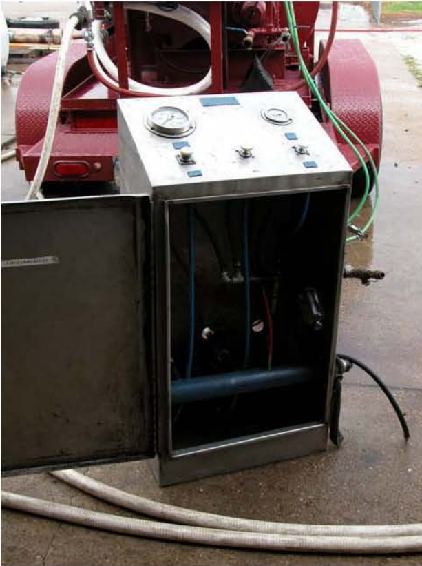
Fig. 14. Control system for Hydrokinetics™ system.
