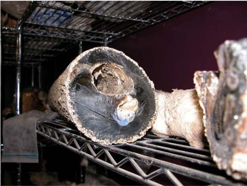
Fig. 11. Solidified line plug removed using Hydrokinetics™.
