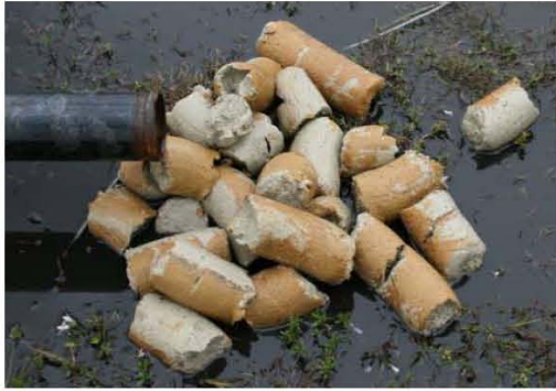
Figure 33. Unplugged 12 ft Bentonite plug after trials with AIMM at 1822 ft pipeline.
