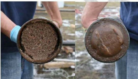
Figure 31. 4 ft Kmag plug after unplugging trials with AIMM. Front side (left) and back side (right).
