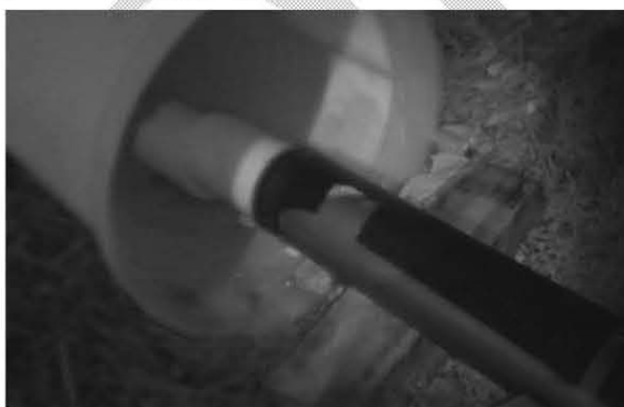
Figure 16. Na-Al-Si plug during extrusion test.
